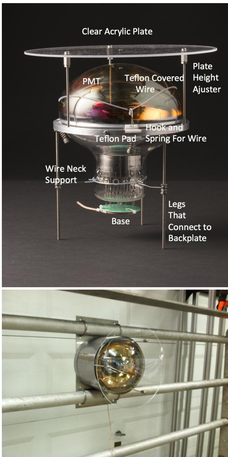
**Figure 35.** Top: the optical unit mount internal to the shield, with components labeled; bottom: unit mounted on rails. The clear plates were replaced with TPB-coated plates immediately before LArTPC installation, as discussed in the text [40, 45].
