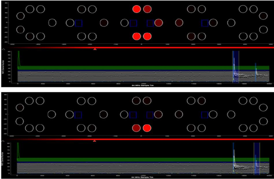
**Figure 27.** Displays showing two sequential events in the argon as seen by the light collection system. The sequence is consistent with a muon that stops (top) and decays (bottom). The circles correspond to the optical units. Red circles indicate those units with hits within the time range indicated by the vertical bars drawn on the PMT waveforms, which are shown at the bottom of each display.
