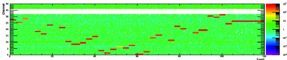
**Figure 40.** Charge detected in each PMT due to flasher tests, shown as a function of time. The y axis is the PMT channel number, the x axis follows the sequencing of signals to the individual PMTs, and the response is given by the color scale. Each PMT is flashed for a short period. The white band indicates unused channels.
