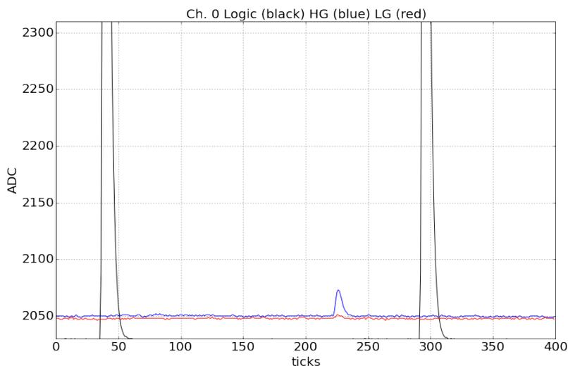
**Figure 43.** Example waveform captured by the PMT readout electronics during single photo-electron calibrations. The black waveforms are logic pulses that mark the time at which an LED in the flasher system is driven. After some delay coming from PMT cable lengths and the flasher system, a candidate single photo-electron pulse is seen (at  $\sim 230$  ticks).
