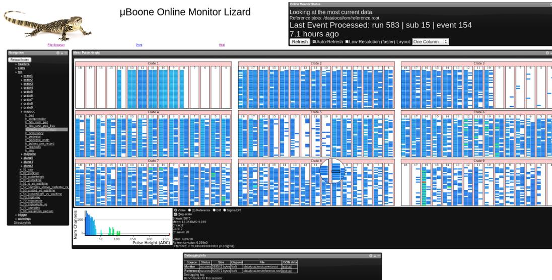
**Figure 64.** The online monitoring GUI (Lizard). The pedestal-subtracted ADC values for all 8256 wires in one minimum bias event are shown. Each box is a channel. Not all crates are fully populated with electronics.
