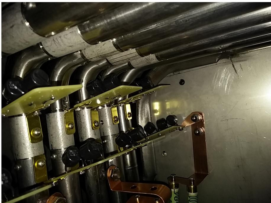
**Figure 16.** Surge-protecting varistors (small black disks in the photograph) are installed in parallel with the voltage divider resistors for the first 32 field cage loops. Here, they are shown mounted on small boards in sets of 3, and attached to the field cage by means of 6-32 hex-head button-screws.
