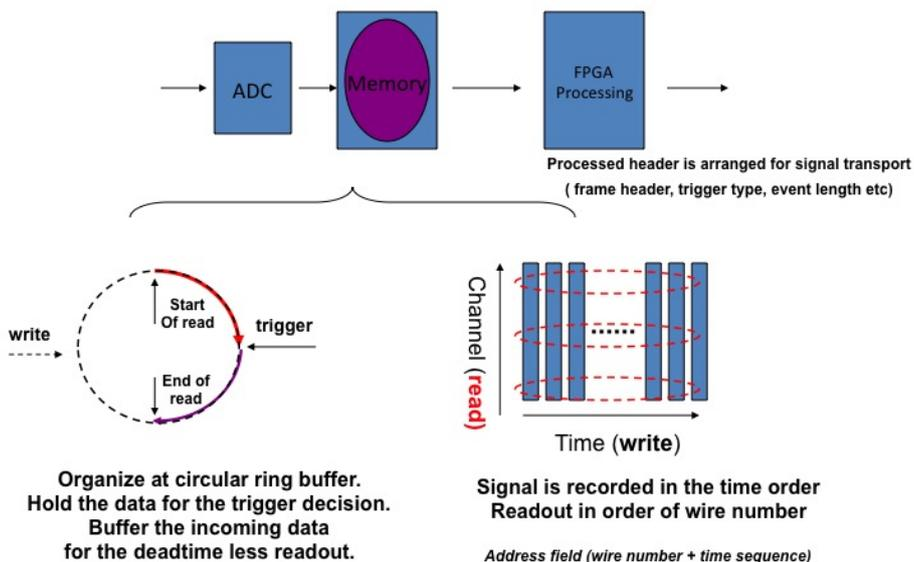
Figure 55. MicroBooNE readout sequence in the TPC FEM.
