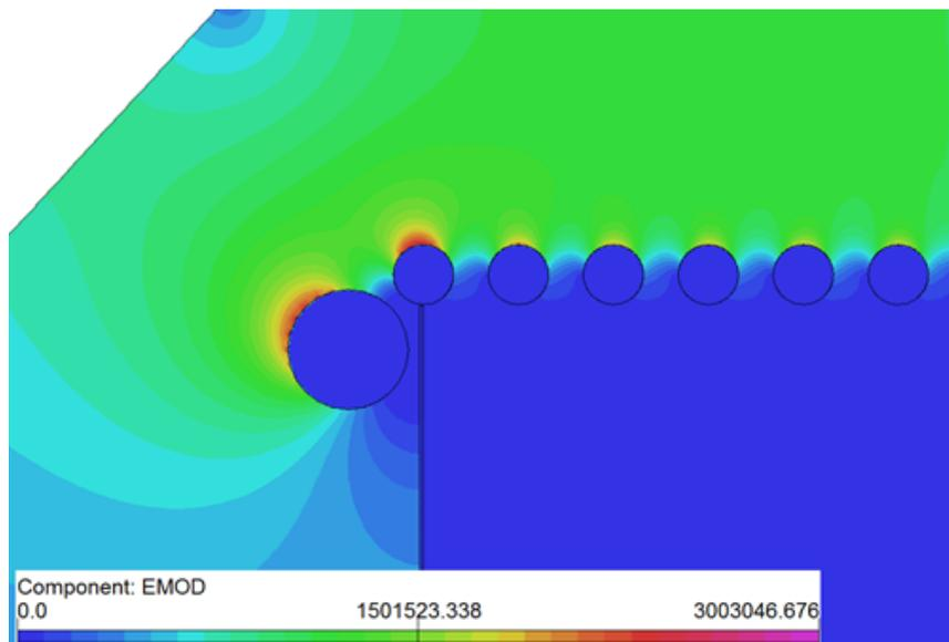
**Figure 13.** Cross-section view showing the electric field simulation inside the field cage when the cathode is set to a voltage of  $-128$  kV. Loop 0 is represented by the larger diameter circle on the left of the image. The legend shows the absolute values of electric field modulus in units of V/m.
