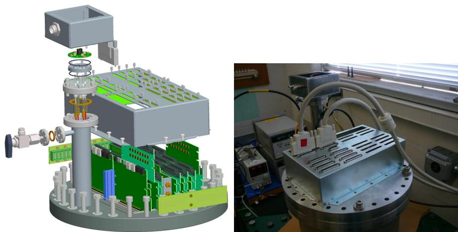
**Figure 51.** Left: diagram of the signal feedthrough assembly, which includes intermediate amplifiers, Faraday cage, bias-voltage feedthrough and filtering circuit. Right: photograph of one of the feedthrough assemblies, partially constructed and being tested.
