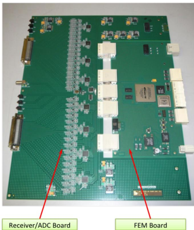
Figure 54. Photograph of a MicroBooNE ADC+FEM board.
