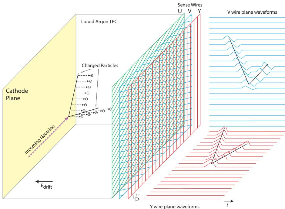
**Figure 2.** Operational principle of the MicroBooNE LArTPC.
