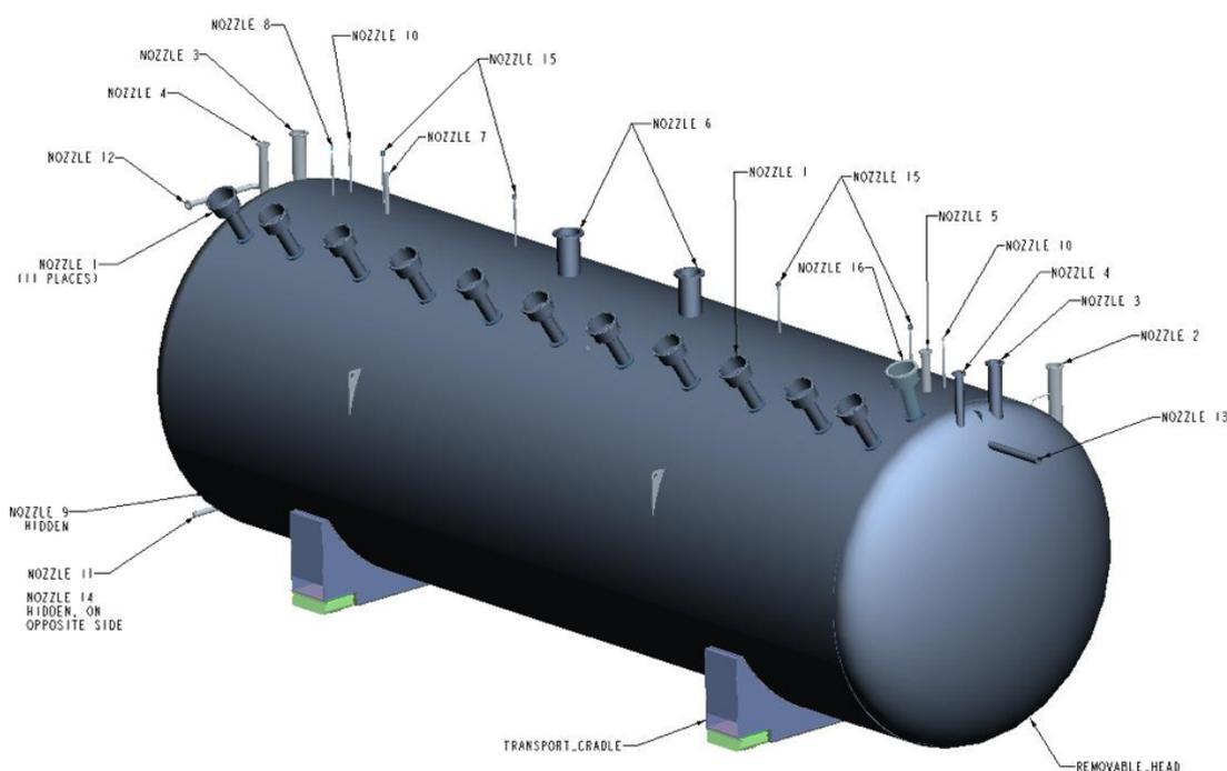
**Figure 5.** MicroBooNE cryostat with nozzle penetrations labeled.
