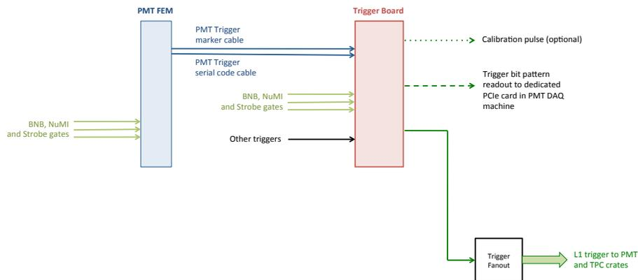
**Figure 60.** PMT readout and trigger logic.
