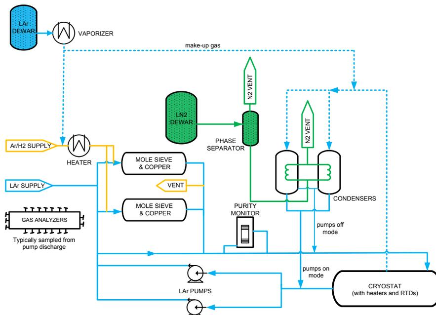
**Figure 7.** Flow diagram of argon in MicroBooNE, showing direction of liquid and gaseous argon in the cryogenic system. Dashed lines represent gas lines, solid lines represent liquid lines, and yellow lines are for the filter regeneration. Gaseous argon from the cryostat is condensed and directed through the purification subsystem. Liquid argon drawn from the cryostat volume is directed into the purification subsystem.
