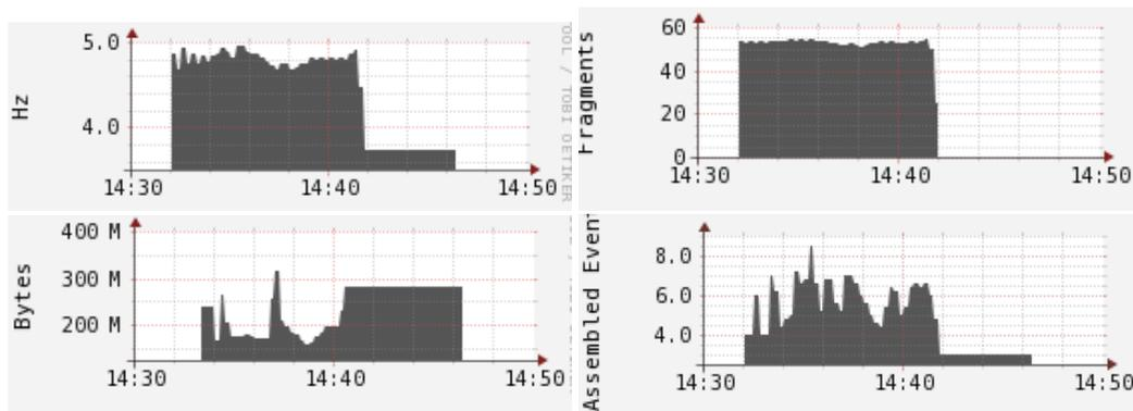
**Figure 63.** Ganglia metrics showing data flow on the EVB machine during a 5 Hz test run. Shown as a function of time are: the external trigger rate (top-left), the received fragment rate (top-right), the disk data write rate (bottom-left), and the number of assembled queued-up events waiting to be written (bottom-right). (11 fragments constitute a complete event in the MicroBooNE DAQ.)
