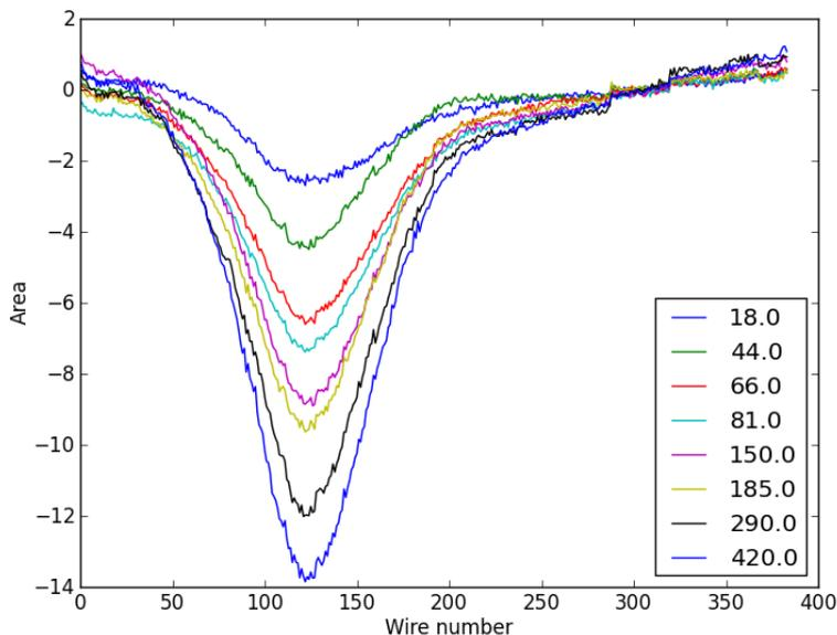
**Figure 41.** Area of signal pulses recorded on collection plane (in arbitrary units) as a function of wire number (arb. offset). The legend indicates the calibrated photo-electron count. The signal pulses are averaged over 50,000 repetitions. The plots are pinned together at wire 300, as the distribution baseline fluctuated over the course of the experiment due to intermittent noise.
