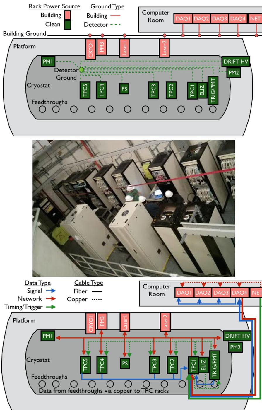
**Figure 65.** Top: diagram illustrating location of deployed electronics racks and separation of detector and building grounds and clean and building power for differing racks. Middle: photograph of installed electronics racks on the LArTF platform. Bottom: a diagram illustrating the general scheme of signal, network, and timing signal cabling in the LArTF computer room and platform.
