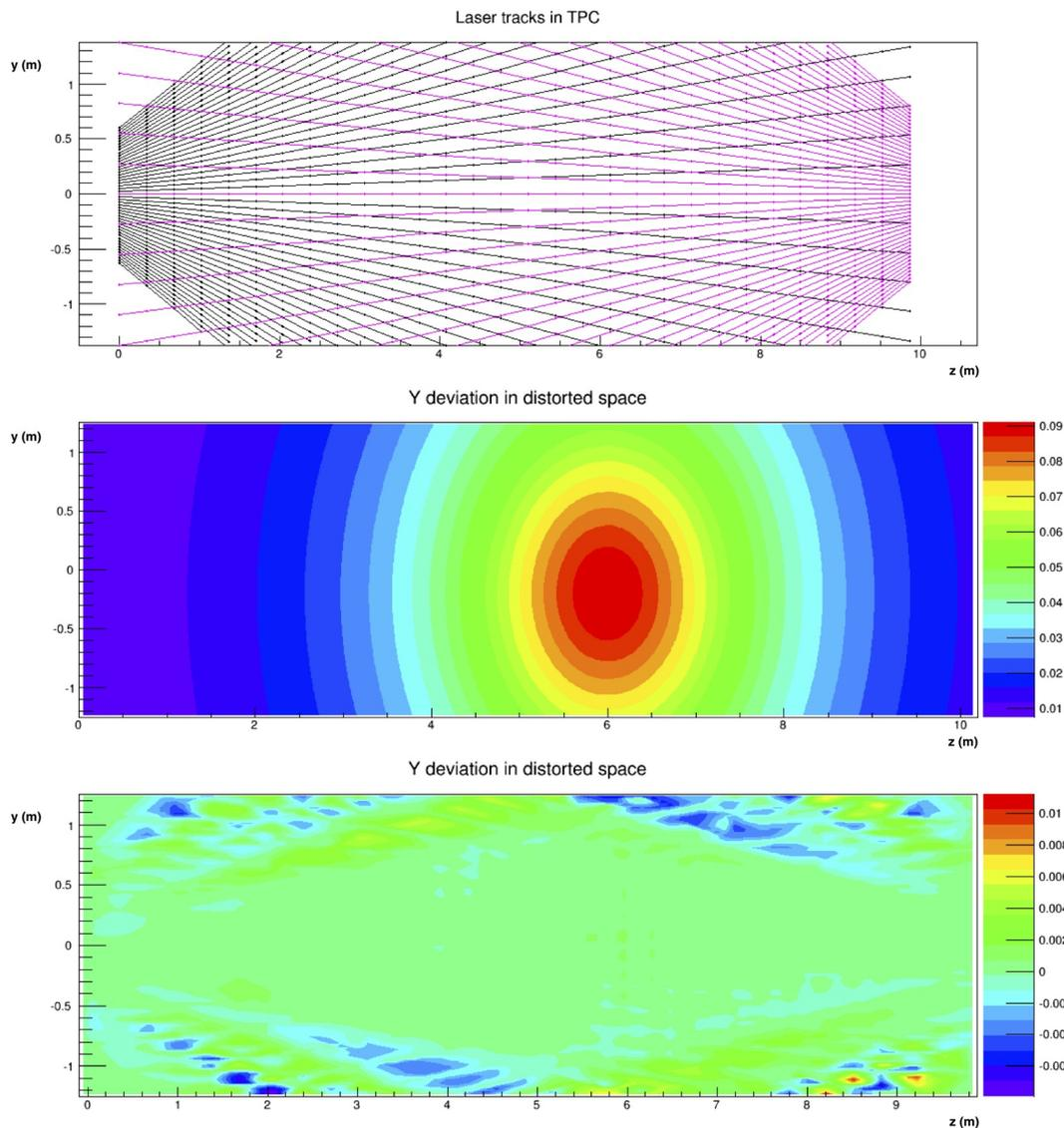
**Figure 73.** Top: simulated true laser beam trajectories in the detector; middle: a map of the discrepancy between reconstructed and true track Y coordinate under influence of non-uniform electric field, as a function of the true Z coordinate of the track; bottom: map of the residual (true - reconstructed) track Y-coordinates, as a function of the true Z coordinate of the track, after applying the UV laser electric field calibration methods.
