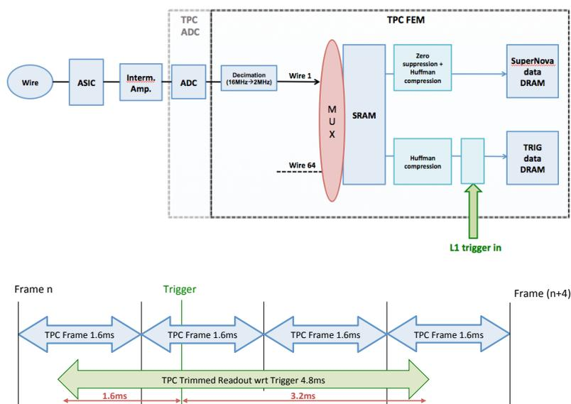
**Figure 56.** MicroBooNE trigger readout.
