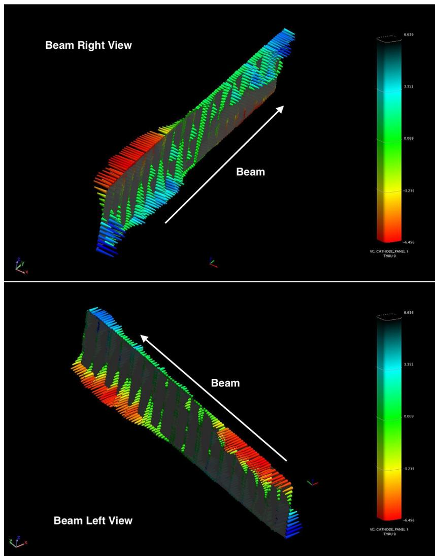
**Figure 11.** Survey results showing the flatness of the cathode, as viewed from the interior (top) and exterior (bottom) sides, after shimming. Color scale extends from  $-6.498$  mm (red) to  $+6.636$  mm (blue).
