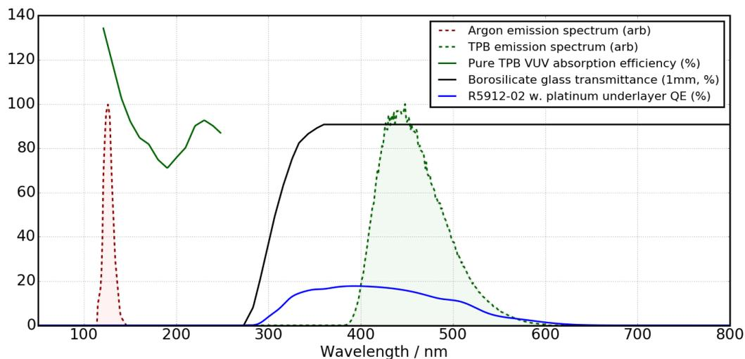
**Figure 28.** Scintillation light emission spectrum (red) and TPB re-emission spectrum (green), in arbitrary units. Superimposed are relevant efficiencies (plotted in % on the y axis): dark green line – absorption of VUV light by TPB; black line – transmission of borosilicate glass; blue line – efficiency of a R5912-02mod cryogenic PMT [50].
