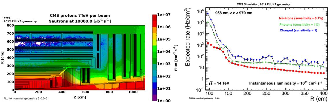
**Figure 10.** Left: Expected neutron flux, in  $\text{Hz}/\text{cm}^2$ , in the Muon system. An  $R$ - $z$  view of one quarter of the CMS detector is shown. Right: Expected rate, from neutrons, photons, and charged particles, as a function of the radial distance from the beamline, for a  $z$  distance between 790 and 802 cm from the IP. The future RE3/1 ring will cover the radial range between 160 and 330 cm.
