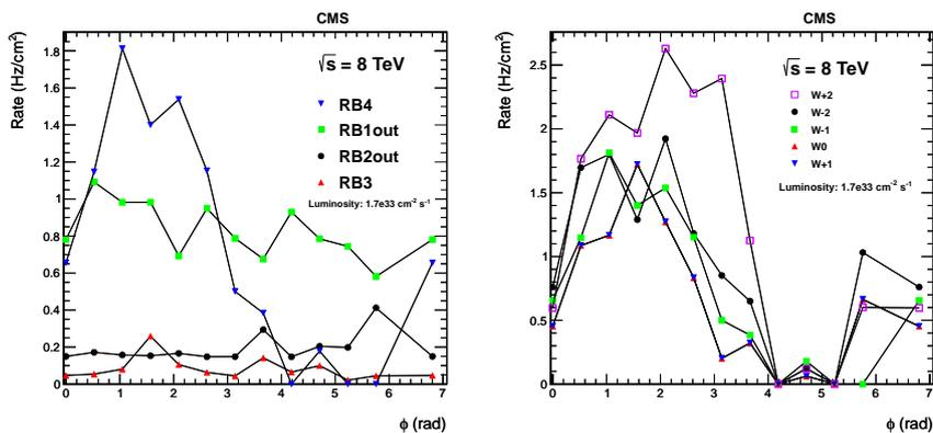
**Figure 6.** Left: Background rates of RPC chambers located in inner and outer layers of the barrel wheel W-1, as a function of the chamber azimuthal position, for a luminosity of  $1.7 \cdot 10^{33} \text{ cm}^{-2} \text{ s}^{-1}$  in 2012. A dependence on the chamber azimuthal position ( $\phi$  asymmetry) is shown for the external layer RB4. Right: Background rates of the RB4 layers in all barrel wheels. The larger rate in the W+2 wheel is discussed in the text.
