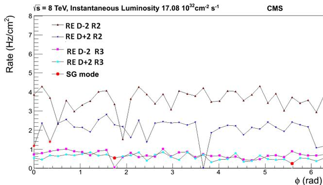
**Figure 7.** Background rates of RPC chambers located in the rings R2 and R3 of the endcap disks D+2 and D-2, as a function of the chamber azimuthal position, for a luminosity of  $1.7 \cdot 10^{33} \text{ cm}^{-2} \text{ s}^{-1}$  in 2012. Note the higher rate in D-2/R2, mentioned in the text.
