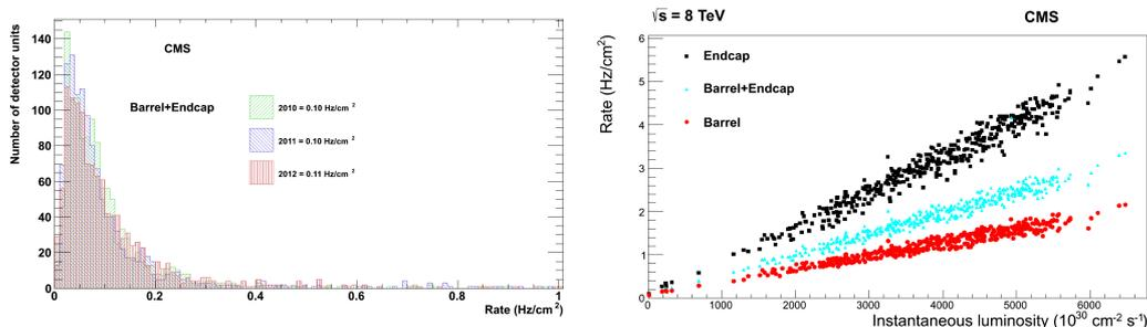
**Figure 3.** Left: average noise rate measured in the whole RPC detector, in 2010 (light green), 2011 (blue), and 2012 (dark red) in absence of pp collisions, during cosmic runs. The average noise level is approximately  $0.1 \text{ Hz/cm}^2$ , constant in time. Right: average background rate as a function of the instantaneous luminosity, measured in 2012 in the RPC barrel (red) endcap (black) and in the total system (barrel plus endcap, shown in light blue).
