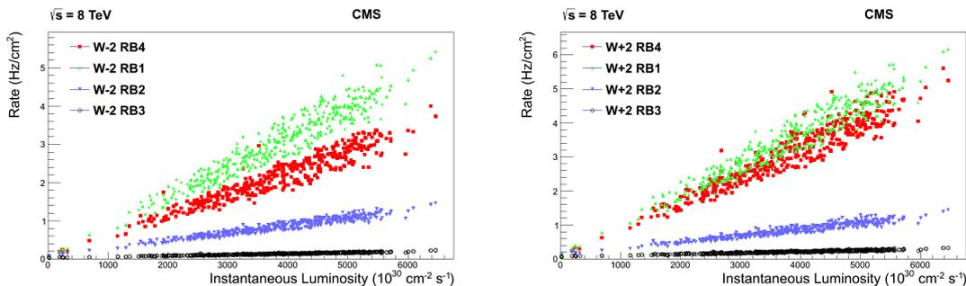
**Figure 4.** Background rate in the radial layers of W-2 (left) and W+2 (right). Larger rates are measured in the innermost (RB1) and outermost (RB4) layers, as discussed in the text. The plus-minus asymmetry of the RB4 layers of the external wheels can also be appreciated from the comparison between the two plots, showing higher background levels on the plus side.
