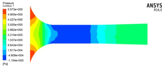
**Figure 9.** Contour pressure of convergent-parallel nozzle.
