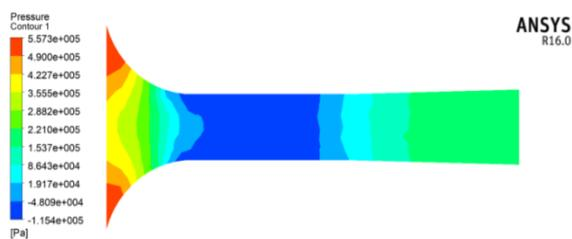
**Figure 7.** Contour pressure of convergent nozzle.
