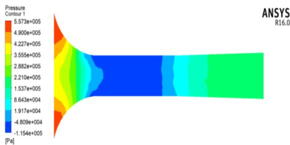
**Figure 5.** Contour Pressure of 3° inclination angle convergent-divergent Nozzle.
