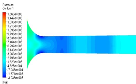
**Figure 3.** Contour of 1° inclination angle convergent-divergent Nozzle.
