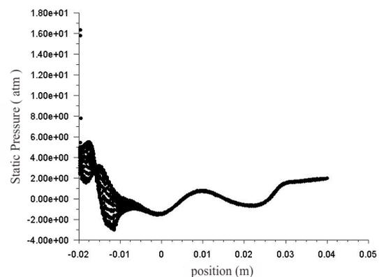
**Figure 4.** Pressure Graph of 1° inclination angle convergent-divergent Nozzle.
