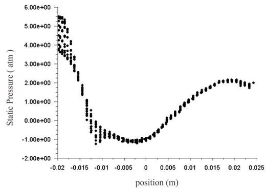
**Figure 6.** Pressure Graph of 3° inclination angle convergent-divergent Nozzle.
