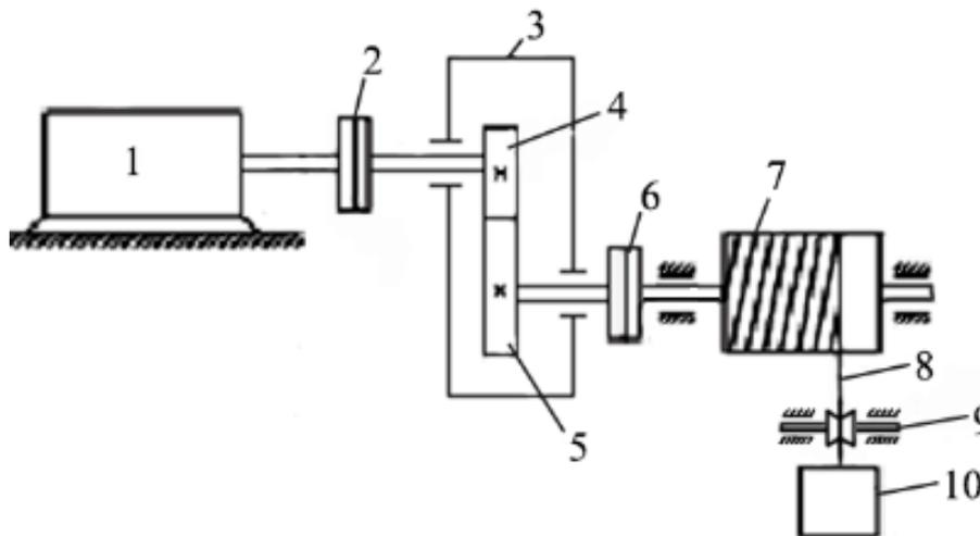
**Figure 1.** A principal scheme of lifting installation: 1 – electric engine; 2, 6 – clutch; 3 – reducer; 4 – gear; 5 – gear wheel; 7 – drum; 8 – rope; 9 – pulley; 10 – lifting vessel.
