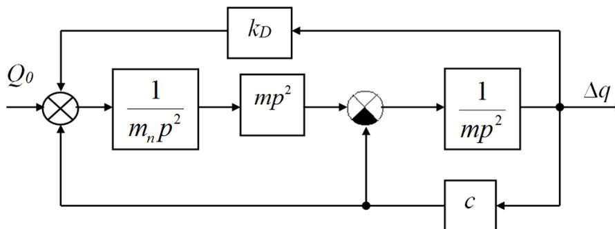
**Figure 3.** Structural scheme of the system with additional feedback on the elastic coordinate
