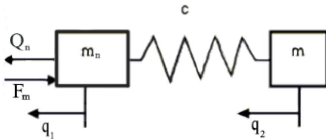
**Figure 2.** Two-mass design scheme of the lifting installation.
