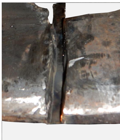
Figure 8. Slotted groove of fractured welded connection with installing a background plate.
