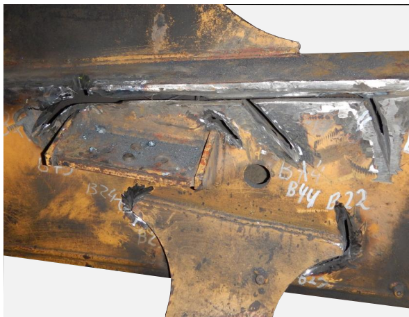
Figure 2. Opening of break on the mine dump truck frame.
