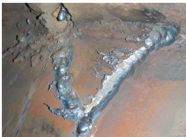
Figure 4. Improper opening of break for making a welding joint.
