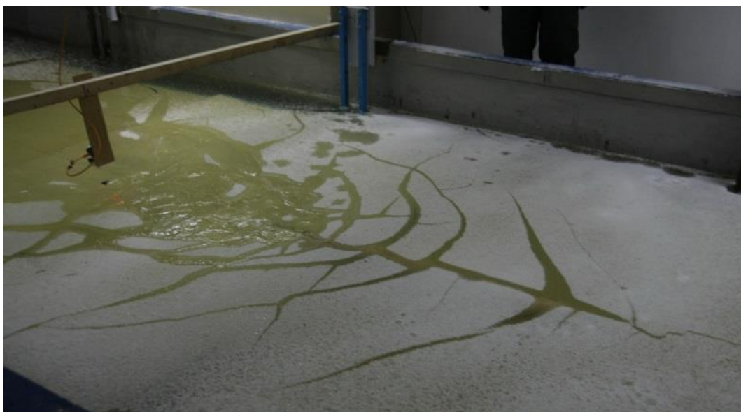
Figure 19. Character of the failure of the model ice by FGW: h_2=0.3 m (the projection №1); u_m=1.78 m/s
