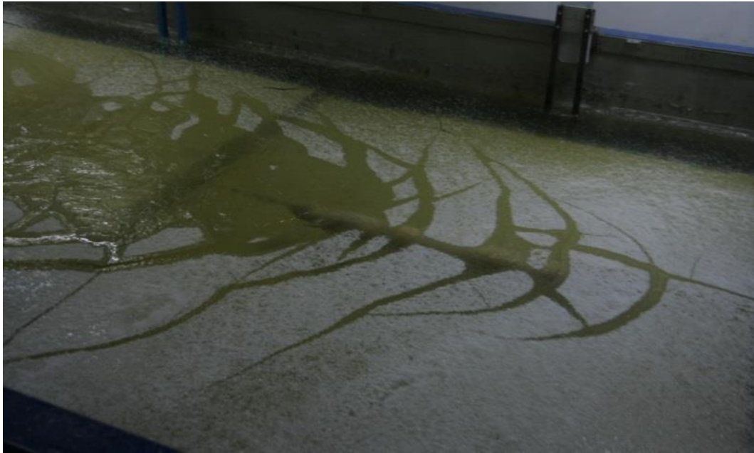
Figure 12. Character of the failure of the model ice by FGW: H_m=0.35 m; h_m=0.16 m; u_m=1.73 m/s
