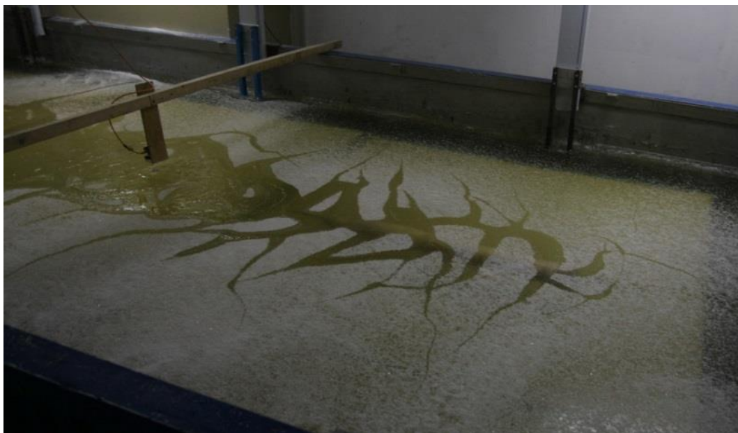
Figure 11. Character of the failure of the model ice by FGW: H_m=0.35 m; h_m=0.16 m; u_m=1.47 m/s
