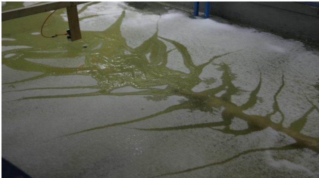
Figure 20. Character of the failure of the model ice by FGW: h_2=0.37 m (the projection №3); u_m=1.62 m/s
