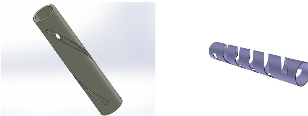
**Figure 6.** X-ray collimator model [8], shown in SOLIDWORKS on the left. On the right is a manually created, proof-of-concept Geant4 model.
