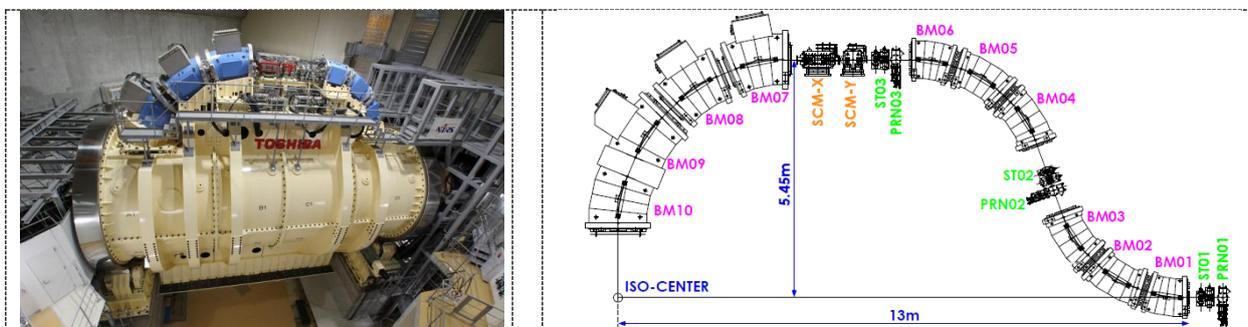
**Figure 1.** Left: Photograph of the rotating gantry at NIRS. Right: Layout of the gantry. The gantry consists of ten superconducting magnets (BM01-10), a pair of scanning magnets (SCM-X and SCM-Y), and three pairs of steering magnets and beam profile-monitors (ST01-03 and PRN01-03).
