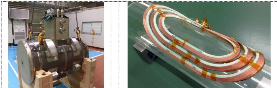
**Figure 6.** Photographs of the HTS model magnet (left) and the saddle-shaped HTS coil (right).
