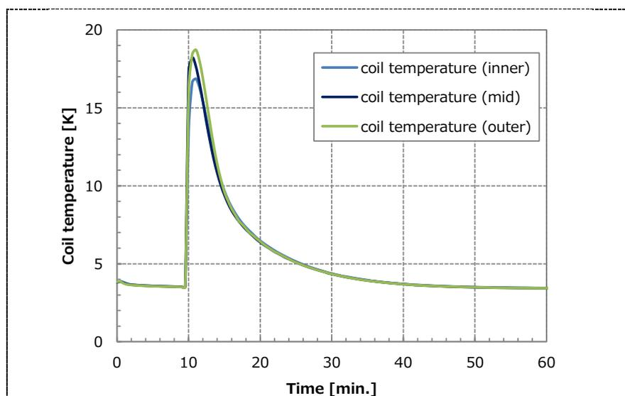
**Figure 4.** The re-cooling curve after quenching was occurred (BM6).
