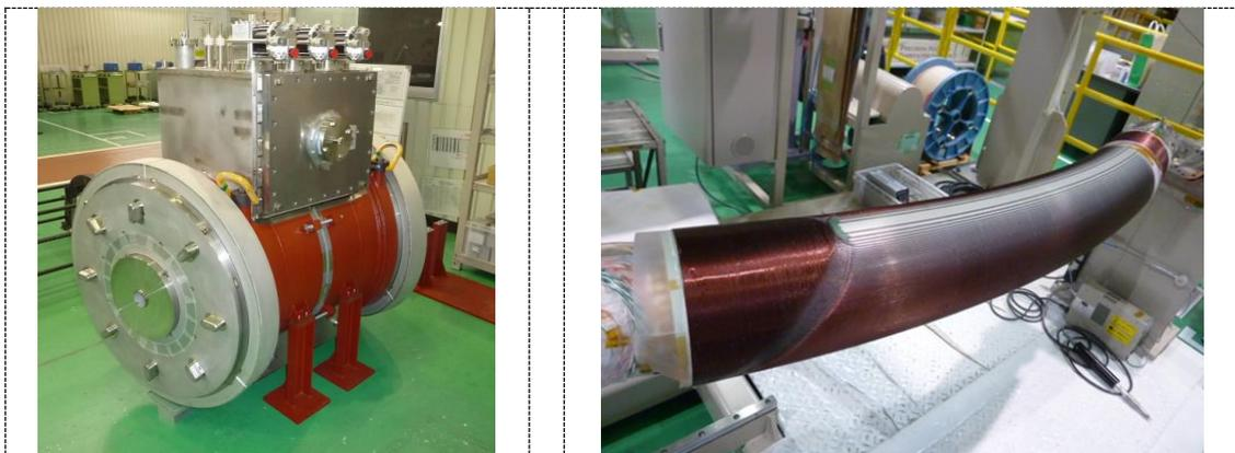
**Figure 2.** Photographs of the LTS magnet (left:BM4) and the saddle-shaped LTS coil (right).
