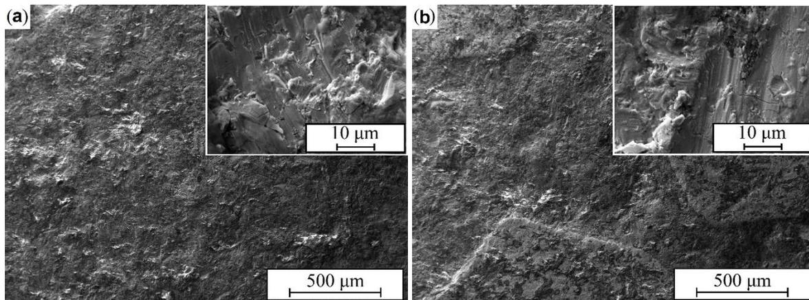
**Figure 9.** Worn surfaces of the hardfacings under high-energy AIEW conditions ( $v = 40$  m/s): a – P1 (unreinforced), b – C5 (50 vol.% angular WC-Co reinforcement).
