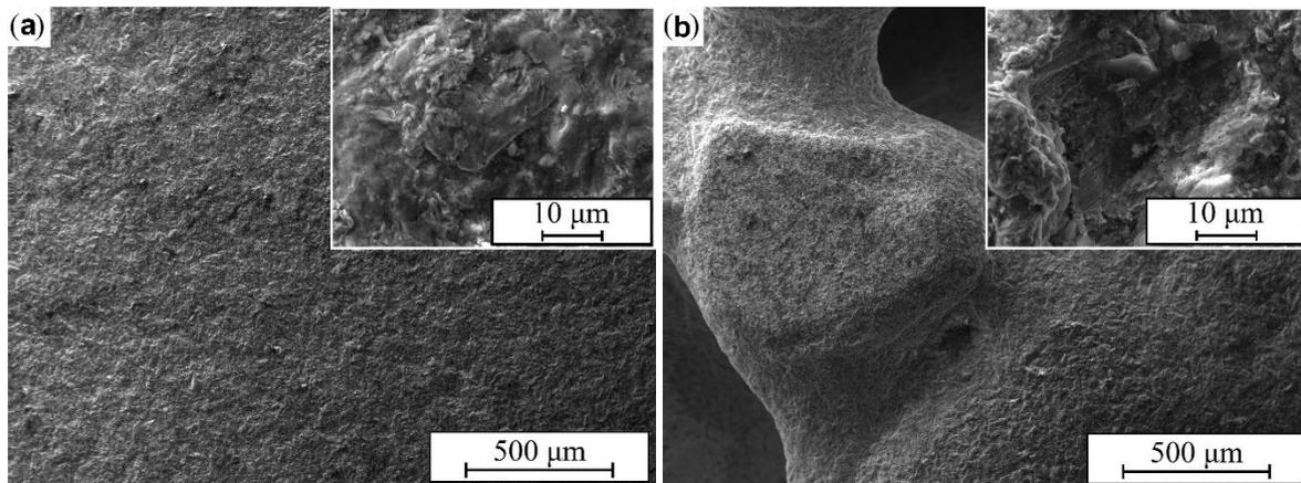
**Figure 8.** Worn surfaces of the hardfacings under low-energy AIEW conditions ( $v = 80$  m/s): a – P1 (unreinforced), b – C5 (50 vol.% angular WC-Co reinforcement).
