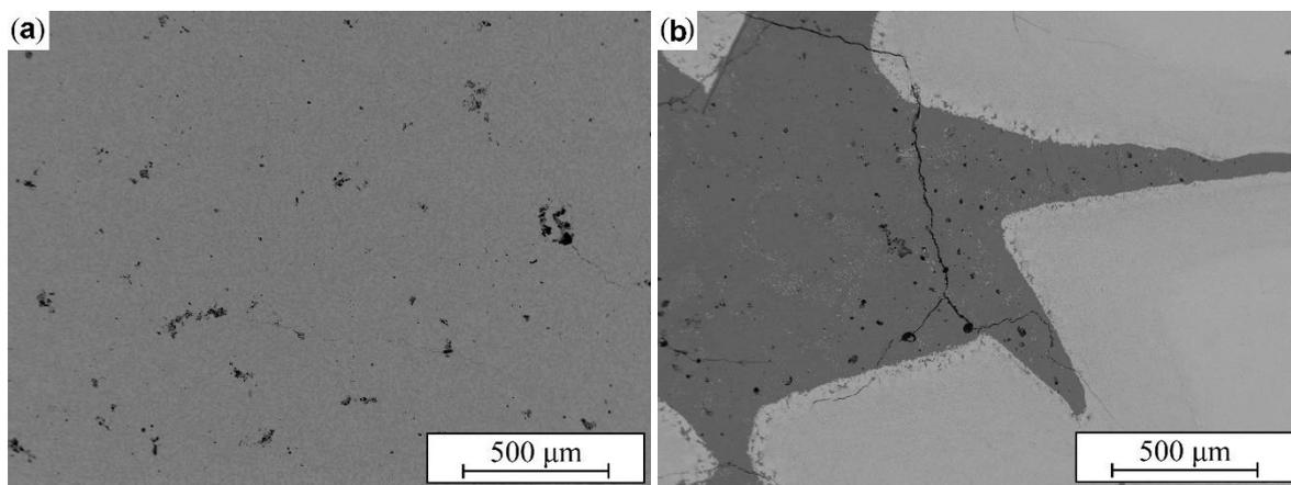
**Figure 1.** Microstructures of the studied hardfacings: a – P1 (unreinforced), b – C5 (50 vol.% WC-Co angular reinforcement) [16].
