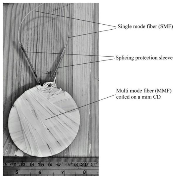
**Figure 1.** The configuration of an SMS fiber structure for vibration sensing.
