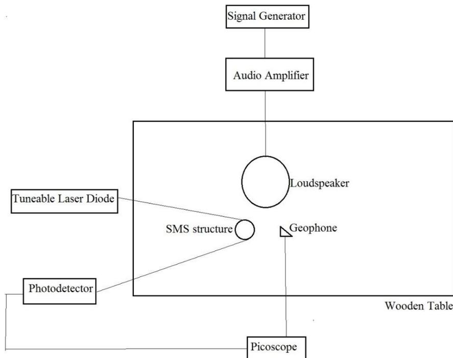
**Figure 2.** Experimental set-up.
