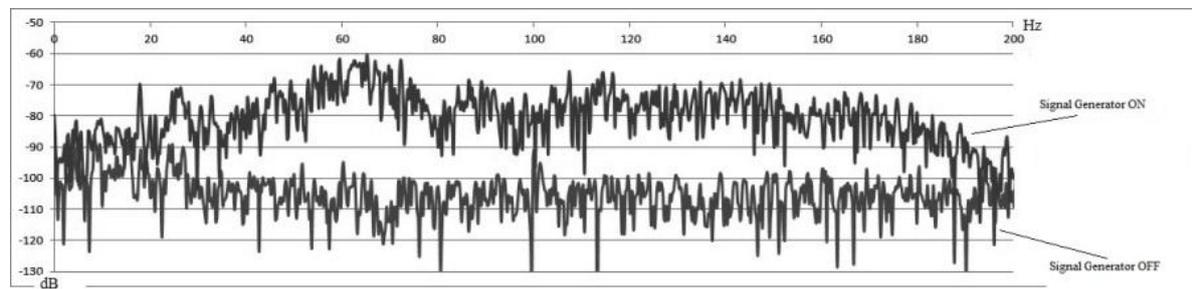
**Figure 6.** Frequency response of the SMS vibration sensor.
