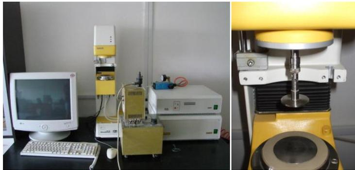
**Figure 3.** Viscometer RS80 and the CP 2Ti 25mm measure head
