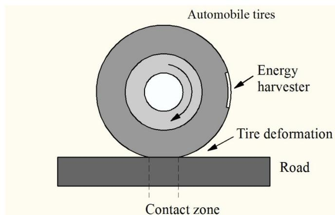
**Figure 3.** The deformation that an automobile tire experiences during a revolution. [38]
