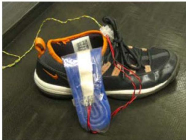
**Figure 4.** A piezoelectric film-based power generator. [39]
