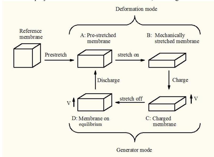
**Figure 2.** Scavenging cycle of a dielectric polymer. [25]
