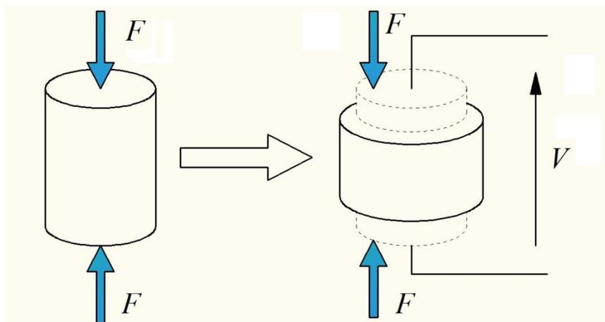
**Figure 1.** Piezoelectric direct effect. [22]
