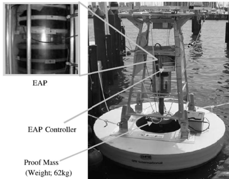
**Figure 5.** EAPs generator system on the test buoy. [29]
