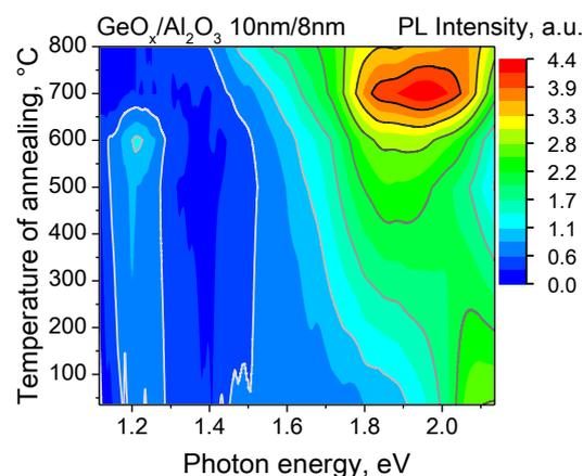
**Figure 7.** PL counterplot of the GeO<sub>x</sub>/Al<sub>2</sub>O<sub>3</sub> nanostructure (10 nm/ 8 nm bilayer) annealed in the temperature range of 500-1000 °C.
