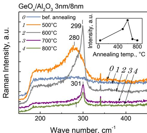
**Figure 4.** Raman spectra of the GeO<sub>x</sub>/Al<sub>2</sub>O<sub>3</sub> nanostructure (3 nm/ 8 nm bilayer) annealed in the temperature range of 500-1000 °C.
