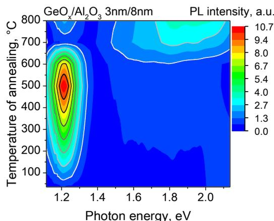
**Figure 5.** PL counterplot of the GeO<sub>x</sub>/Al<sub>2</sub>O<sub>3</sub> nanostructure (3 nm/ 8 nm bilayer) annealed in the temperature range of 500-1000 °C.
