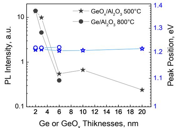
**Figure 9.** The  $1.2\text{ eV}$  PL peak properties.
