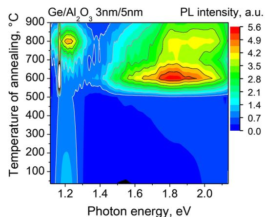
**Figure 3.** PL counterplot of the  $\text{Ge}/\text{Al}_2\text{O}_3$  nanostructure (3 nm/5 nm bilayer) annealed in the temperature range of 500-1000 °C.
