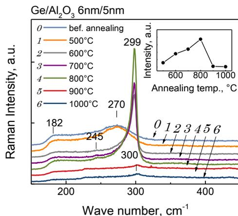
**Figure 2.** Raman spectra of the  $\text{Ge}/\text{Al}_2\text{O}_3$  nanostructure (3 nm/5 nm bilayer) annealed in the temperature range of 500-1000 °C.
