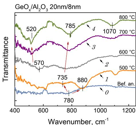
**Figure 6.** FTIR spectra of the GeO<sub>x</sub>/Al<sub>2</sub>O<sub>3</sub> nanostructure (20 nm/ 8 nm bilayer) annealed in the temperature range of 500-1000 °C.
