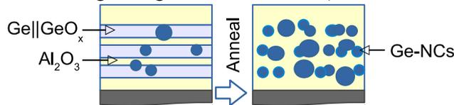
**Figure 1.** Schematic representation of the  $\text{GeO}_x/\text{Al}_2\text{O}_3$  nanostructure modification.
