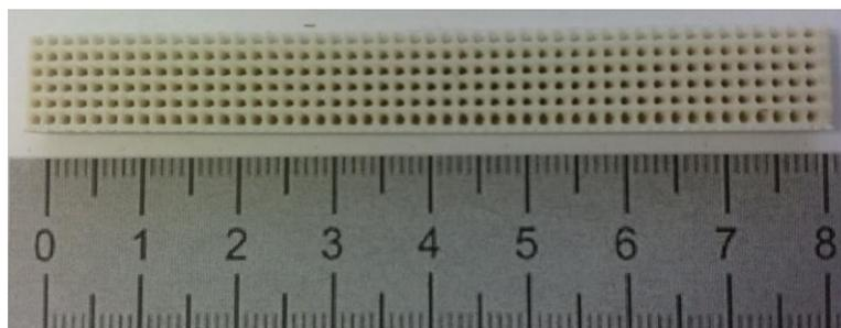
**Figure 2.** 3D-printed scaffold for three-point flexural test
