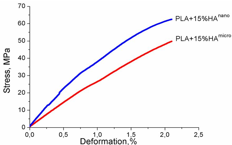
**Figure 4.** Typical stress-deformation curves of compression test for PLA-based composites
