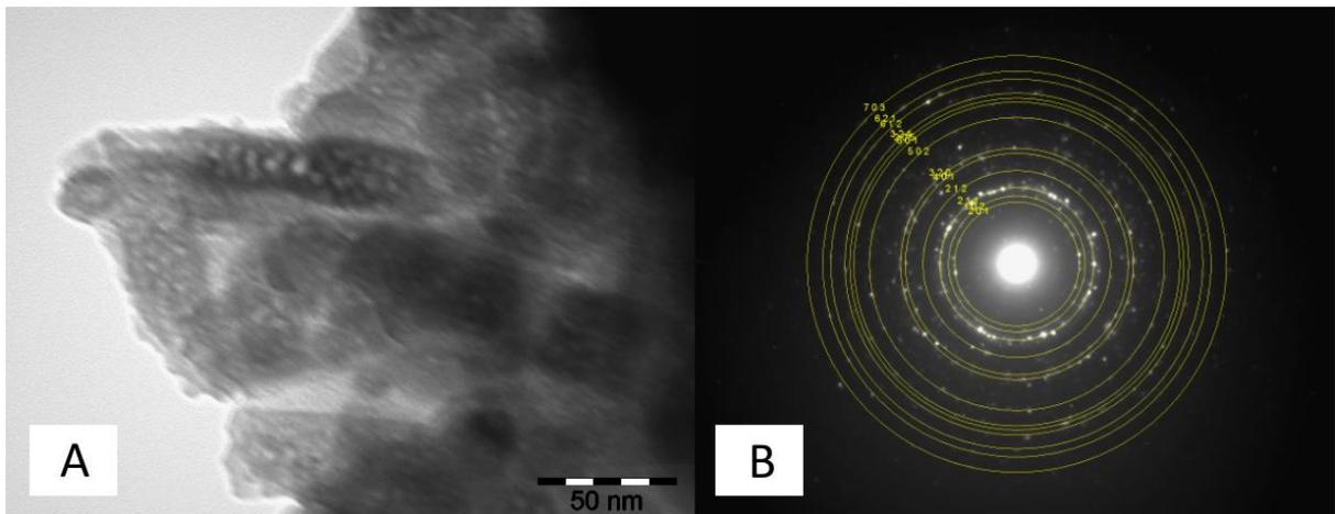
**Figure 3.** TEM image (A) and electron diffraction pattern (B) of HA nanoparticles
