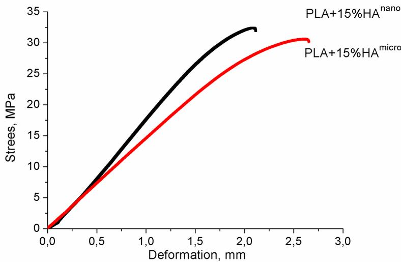
**Figure 5.** Typical three-point flexural curves for PLA-based composites
