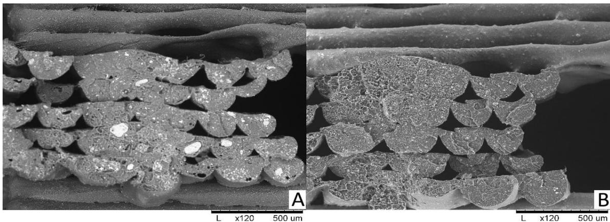
**Figure 6** –SEM imager of fracture surface of PLA-based scaffold after three-point flexural test
