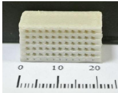
**Figure 1.** 3D-printed scaffold based on bioactive nanocomposite PLA/HA
