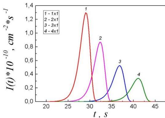
**Figure 1.** Time dependence of nucleation rate for elongated islands with  $r = 1.4$  in Ge/Si(001) system at substrate temperature  $T = 470$  °C and deposition rate  $V = 0.1$  ML/s.
