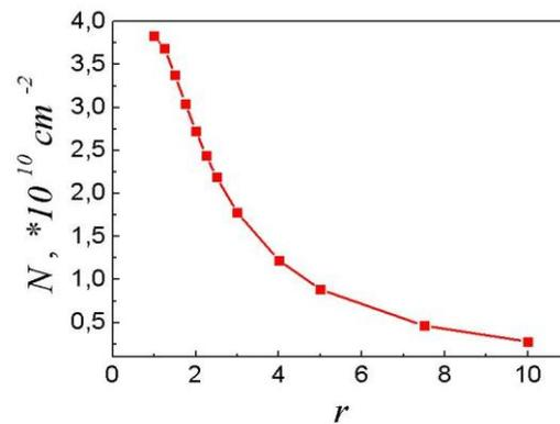
**Figure 2.** Surface density of wedge-like clusters of Ge on Si(001) surface as a function of  $r$  at substrate temperature  $T = 470$  °C and deposition rate  $V = 0.1$  ML/s.
