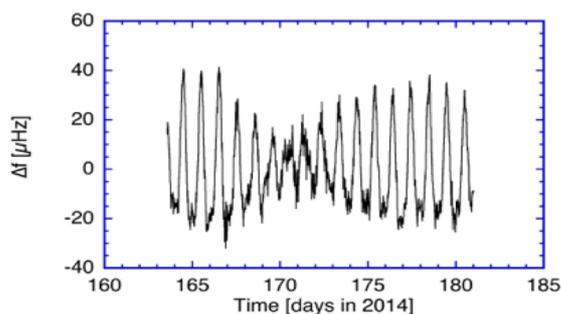
Figure 1: Fluctuation of the Earth rotational rate due to Diurnal polar motion and solid Earth tides, as observed by the laser gyroscope G at the Geodetic Observatory in Wettzell (Bavaria)
