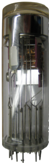
Figure 2. Hamamatsu R7525 – The original HF PMT
