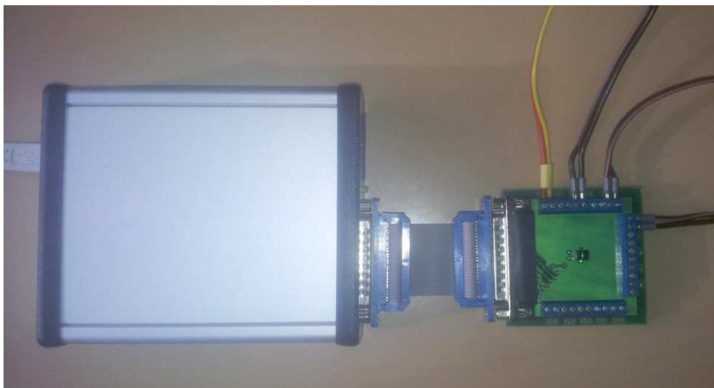
Figure 5. USB module with isothermal terminal block
