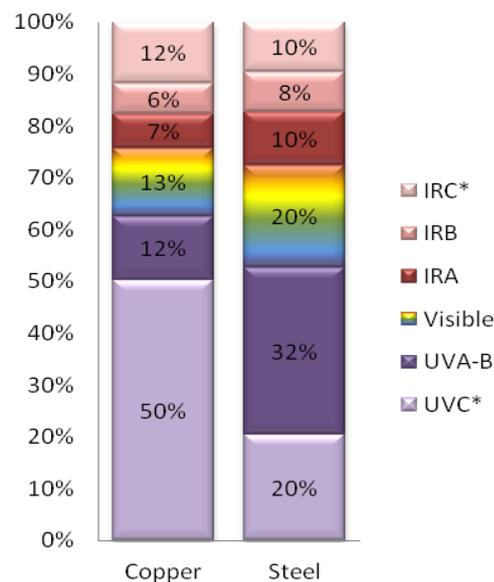
**Figure 3.** Detailed spectral distribution of the measured radiated energy vs the type of electrodes, for the short arc
