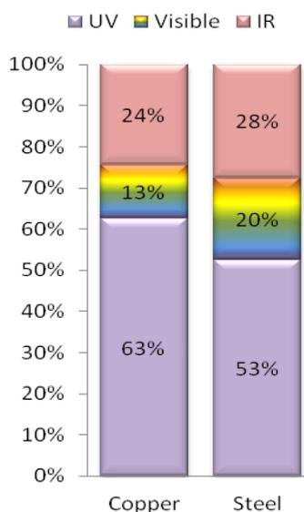
**Figure 2.** Spectral distribution of the measured radiated energy vs the type of electrodes, for the short arc.
