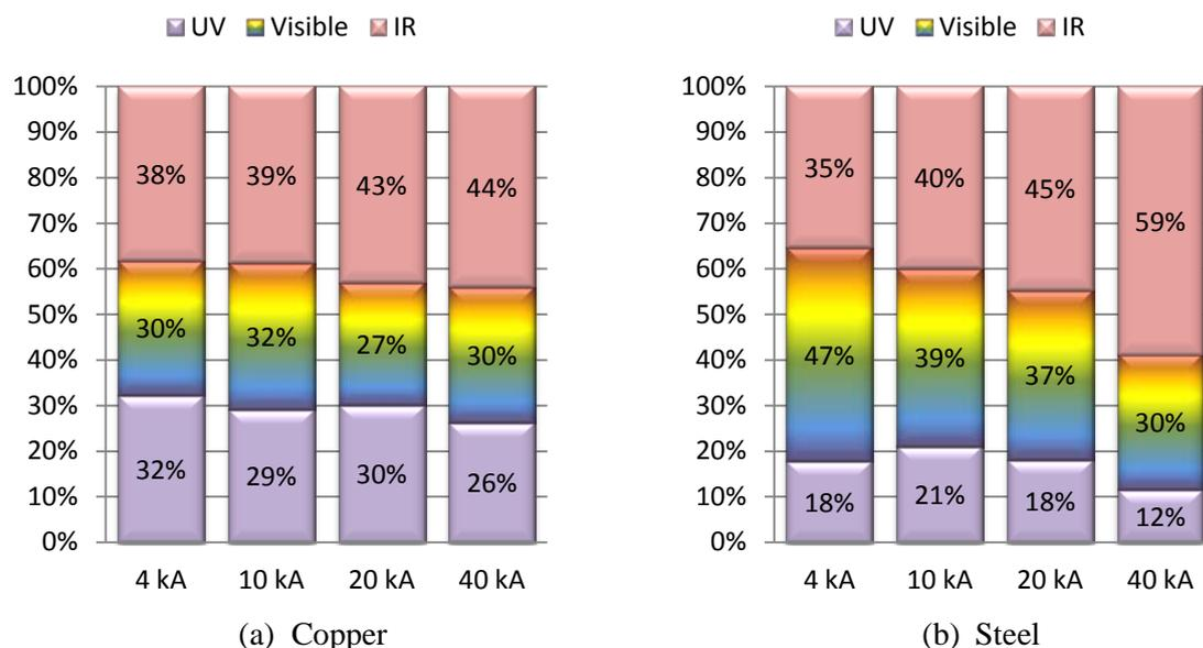
**Figure 4.** Spectral distribution of the measured radiated energy vs the type of electrodes and the current, for the long arc.
