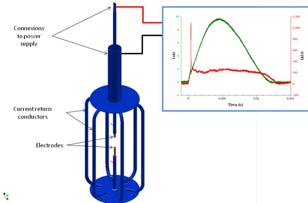
**Figure 1.** Device for the creation and study of the short arc. Typical electric current (green) and voltage (red) curves are shown.
