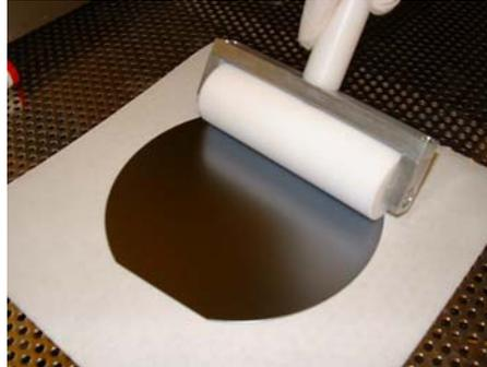
**Figure 3. Imprinting of the SU8 layer from a dummy wafer (6") to the Teflon cylinder.**
