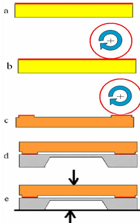
**Figure 2. a) Spinning of SU8-5 photoresist on a dummy wafer, b) contact imprinting of SU8-5 photoresist on a Teflon cylinder, c) imprinting of SU8 from the Teflon cylinder on the wafer surface, d) alignment and contact, e) wafer-to-wafer bonding.**
