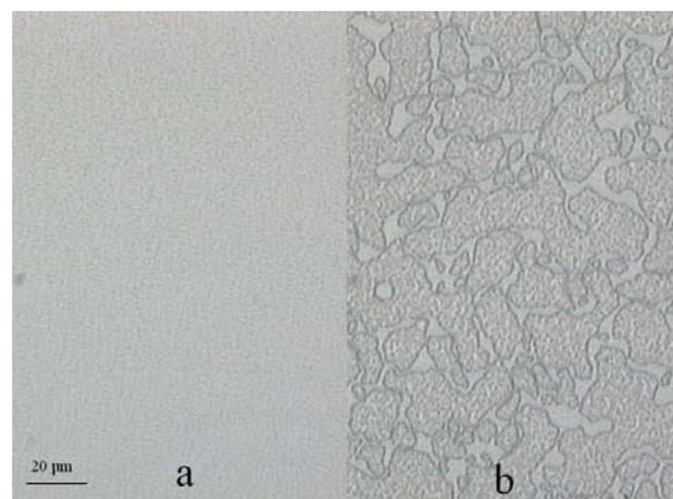
**Figure 5. a) Fully bonded area and b) partially bonded area.**
