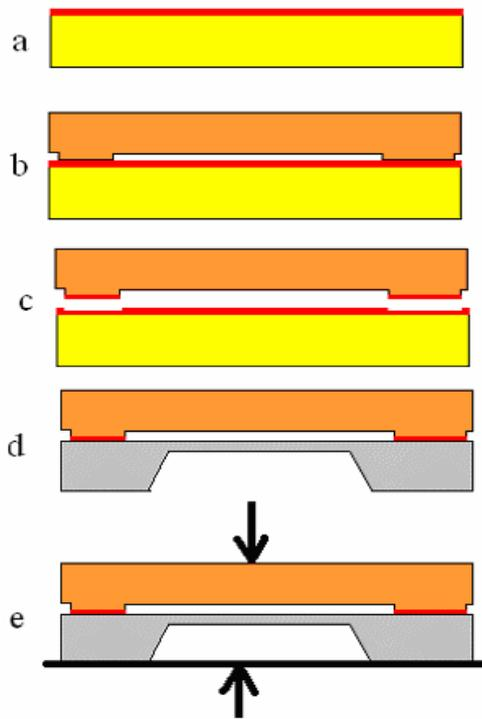
**Figure 1. a) Spinning of SU8-5 photoresist on a dummy wafer, b) contact imprinting of SU8-5 photoresist by attachment of cover wafer on the dummy wafer, c) detachment of cover wafer d) alignment and contact, e) wafer-to-wafer bonding.**
