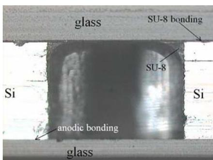
**Figure 6. Microfluidic channel with bulk silicon walls and glass as ceiling and floor.**
