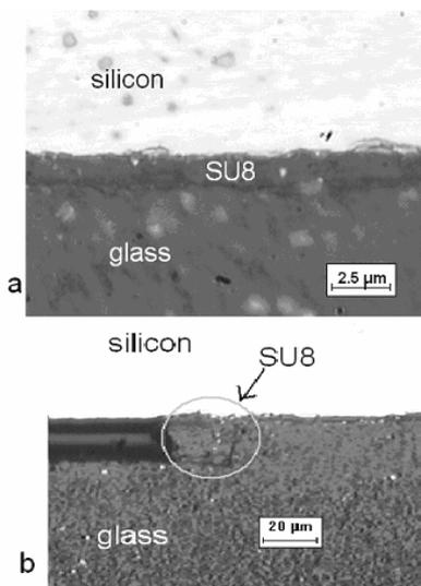
**Figure 4. Optical image with cross s**
