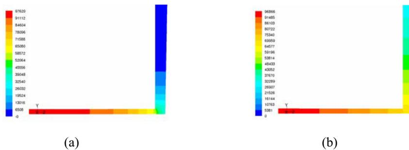
Figure 6. Contours of total-surface-heat-flux-W/m<sup>2</sup> (a) PDC-HWA (b) Platinum-HWA
