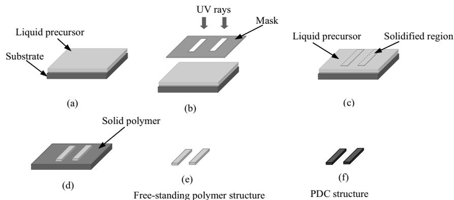
Figure 5. General Fabrication process: (a) spin precursor onto substrate; (b) UV exposure; (c) solidified polymer with remaining liquid; (d) removing non-solidified precursor; (e) remove polymer structures from substrate; (f) crosslink and pyrolyze polymer to obtain PDC structure.
