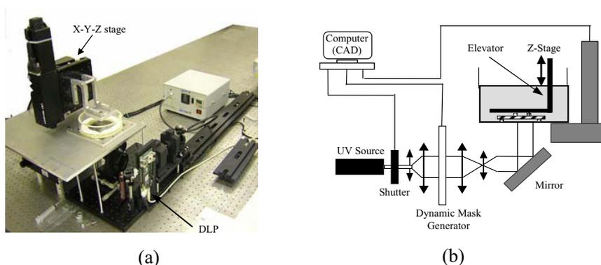
Figure 4. (a) Photograph of Invert-micro-stereolithography developed at UCF and (b) Principle of Invert -  $\mu$ SL
