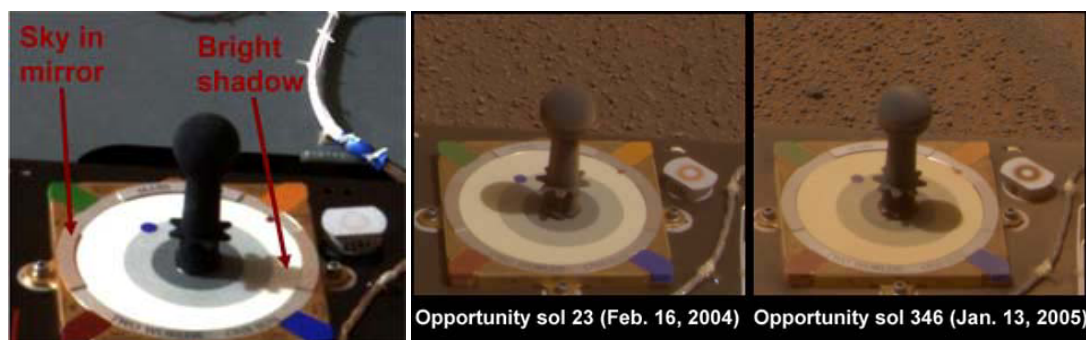
Figure 10. (Left): Clean color calibration target on Mars Exploration Rover Spirit. The target's mirror and the shadows cast on it by the Sun help scientists determine the degree to which dusty Martian skies alter the panoramic camera's perception of color. (Center): Calibration target on the missions' twin rover Opportunity after 23 Martian days (sol). Right): Target after 346 sols. [Courtesy NASA/JPL/Cornell University]
