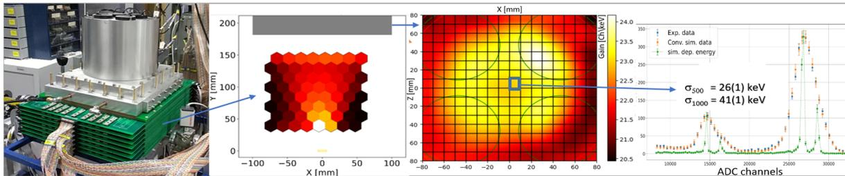
**Figure 1.** The miniBETA spectrometer with beta sources located in the middle of the chamber. (a) photograph of the setup, (b) illumination of the chamber with the cell colors indicating density of hits, (c) gain map of the plastic scintillator and (d) sample of measured  $^{207}\text{Bi}$ -spectrum used for calibration.
