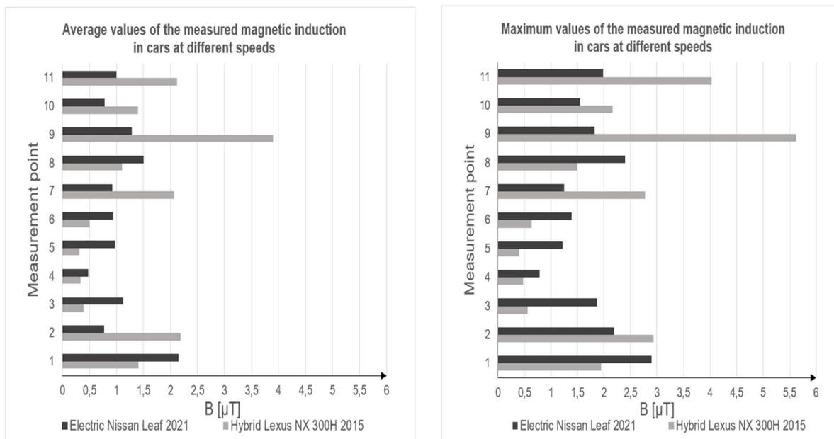
Figure 3. Graphs of average and maximum values of magnetic induction from measurements made at the cockpit of vehicles
