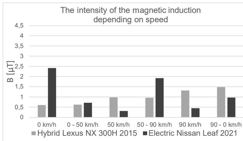
Figure 4. Magnetic induction intensity against speed measured in the driver's seat at abdominal level
