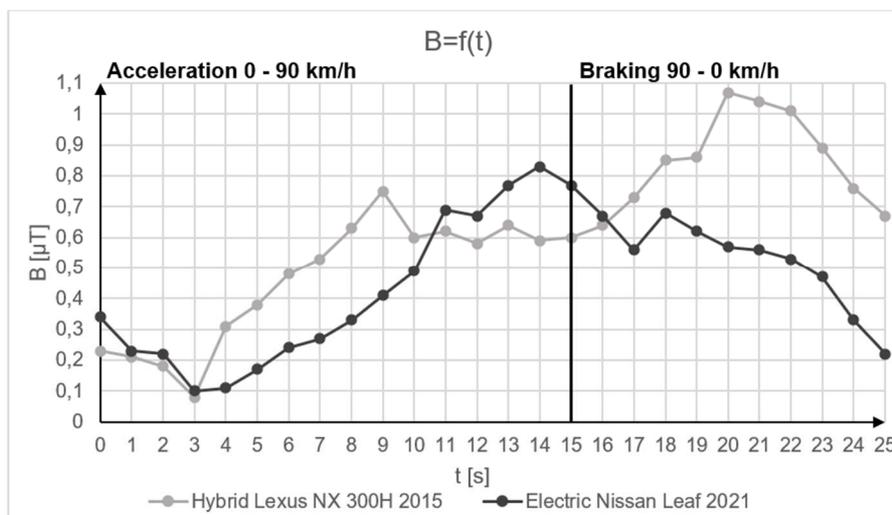
Figure 7. Graph of magnetic induction versus time during acceleration and braking of vehicles. Abdominal measurement in the middle rear passenger seat.
