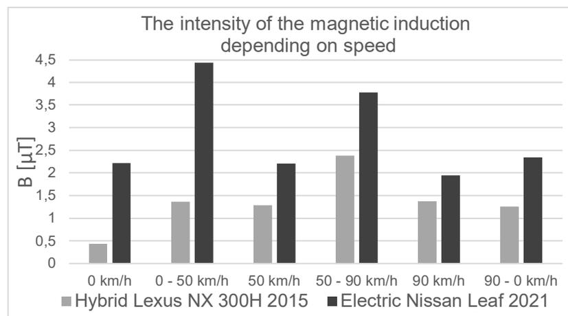
Figure 5. Magnetic induction intensity against speed measured in the middle rear seat at abdominal level
