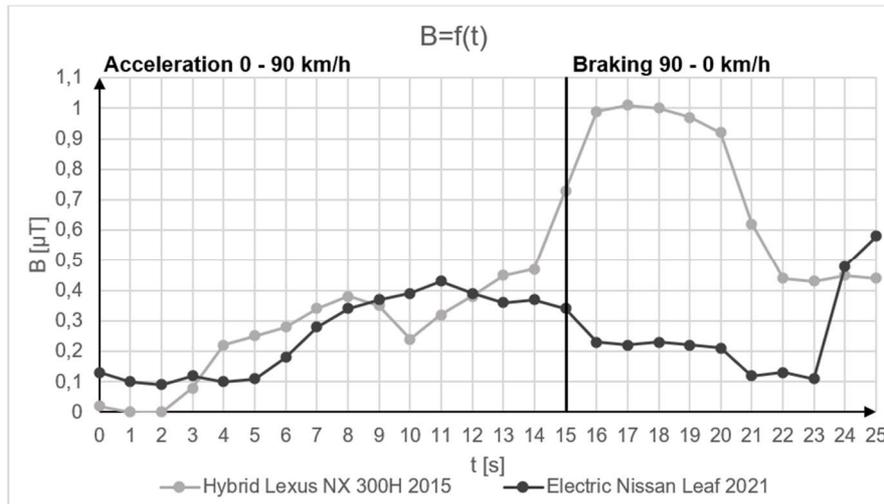
Figure 6. Graph of magnetic induction versus time during acceleration and braking of vehicles. Abdominal measurement in the driver's seat.
