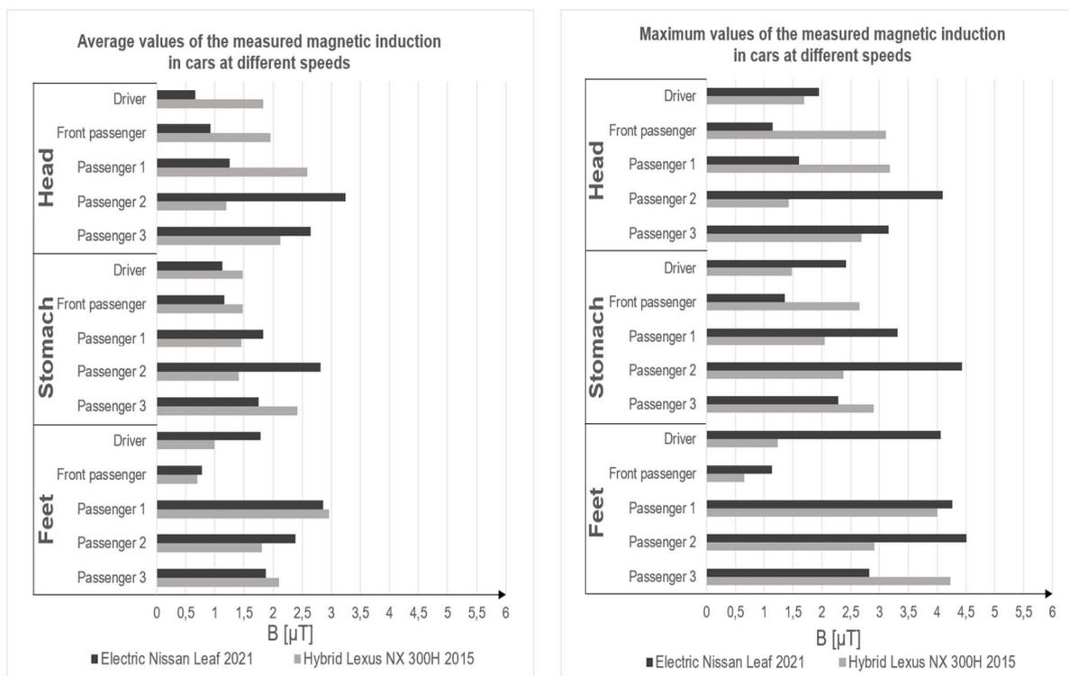
Figure 1. Graphs of average and maximum values of magnetic induction from measurements made in the vehicle cabin on the passenger and driver seats
