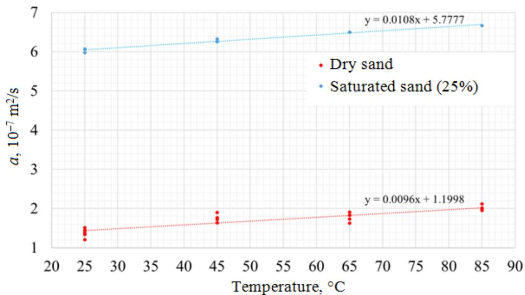
**Figure 5.** Measurement of the thermal diffusivity of dry and moisture-saturated sieved sand as a function of temperature.
