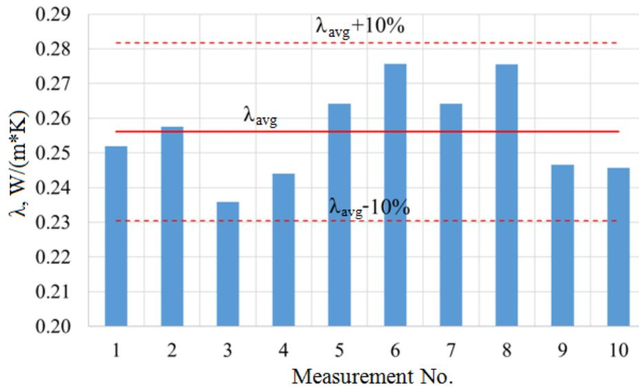
**Figure 4.** Series of measurements of the thermal conductivity of dry sand.
