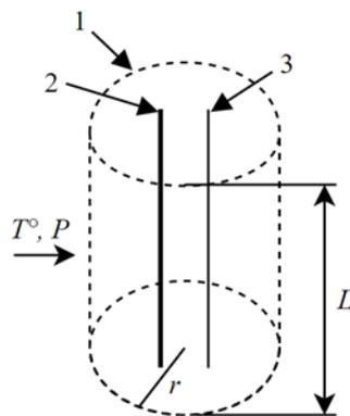
**Figure 1.** Schematic diagram of the linear source method: 1 - rock sample under study; 2 - emitting probe with a linear heat source and a temperature sensor; 3 - receiving probe with a temperature sensor.
