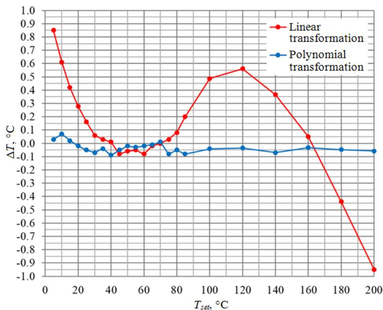
**Figure 3.** Temperature measurement error depending on the type of thermocouple EMF-to-temperature conversion.
