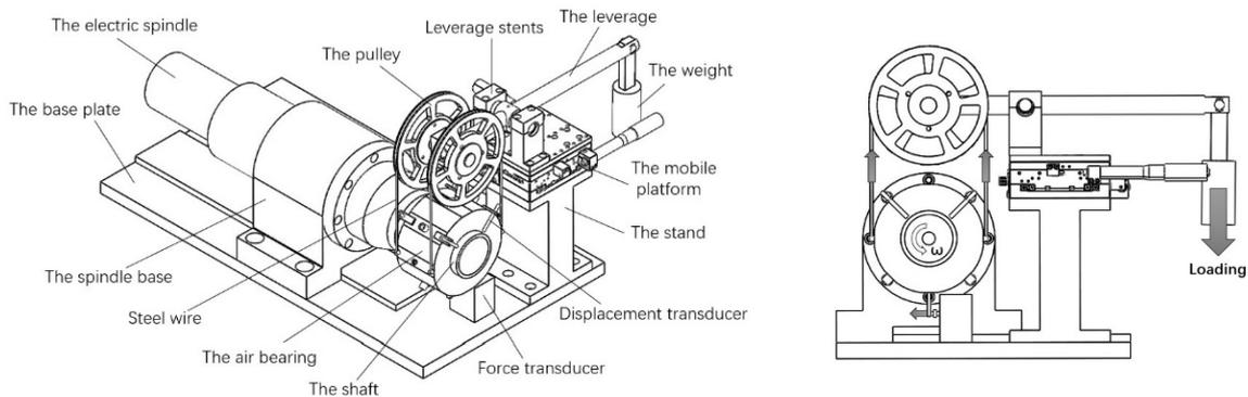
(a) Bearing testing machine structure
