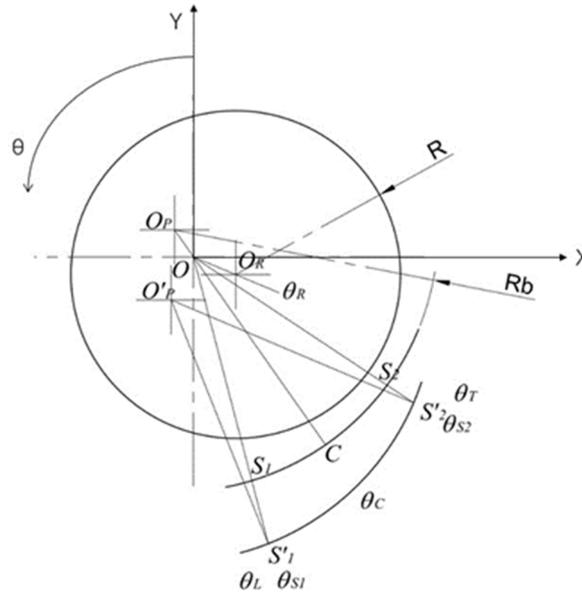
Fig.2 Bearing analysis model
