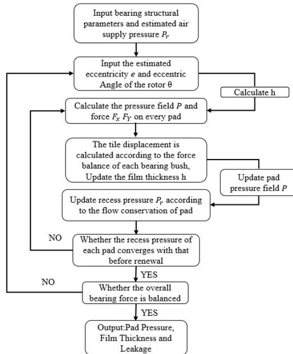
Fig.3 Flow chart of bearing performance prediction calculation
