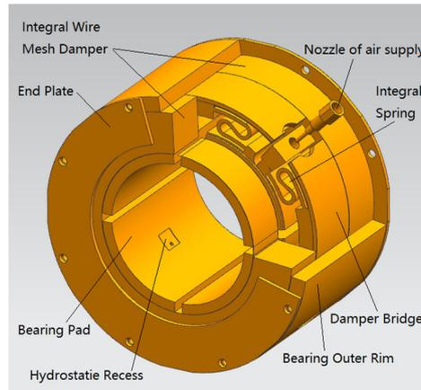
Fig.1 3D structure drawing of bearing
