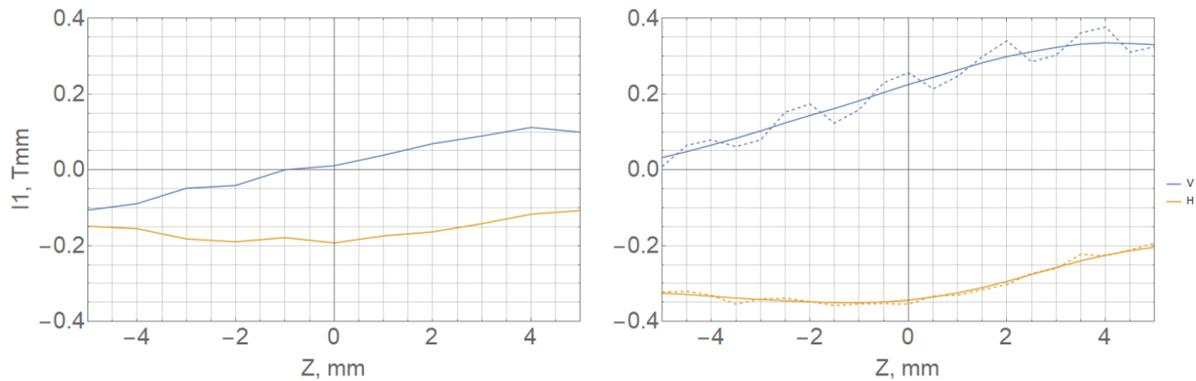
**Figure 3.** First field integral vs transverse position from measurements of the assembled prototype structure (left) and from simulations based on measurements of the individual keepers (right). Blue: vertical component, yellow: horizontal component. The dashed lines in the graph on the right show some systematic errors of the measurement system which is visible only when 32 individual measurements are summed up for prediction.
