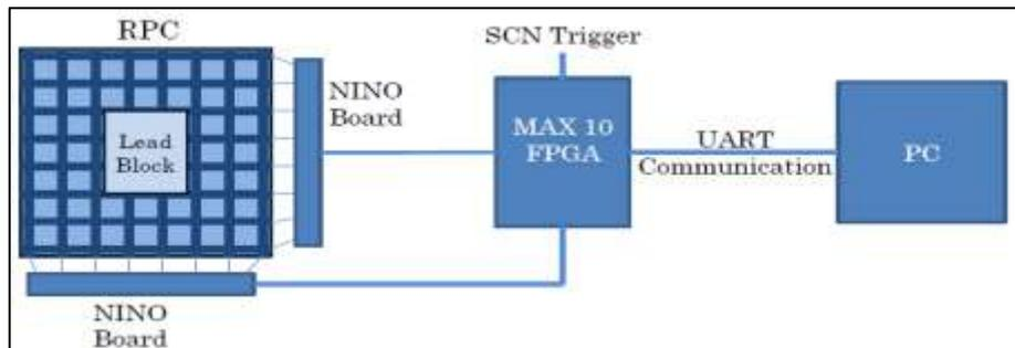
**Figure 7.** Schematic diagram of the test setup for FPGA based DAQ
