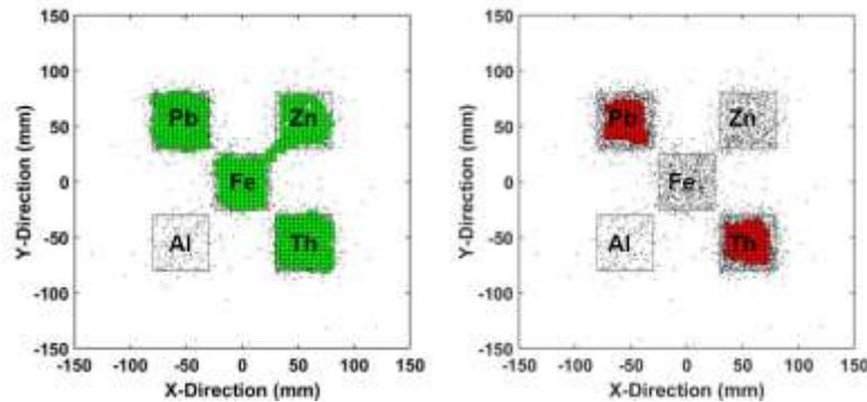
**Figure 3.** The PRM processed images using iron (left) and lead (right) filters
