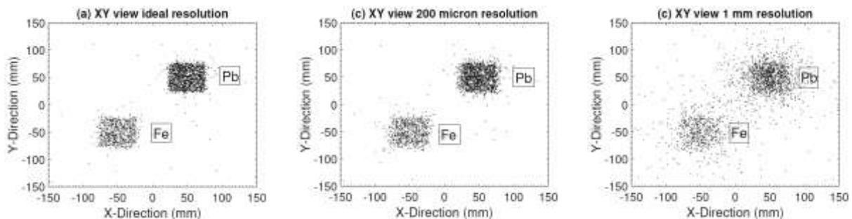
**Figure 2.** The two dimensional images produced by the projection of scattering vertices on the central XY plane with ideal, 200 micron and 1mm detector resolution
