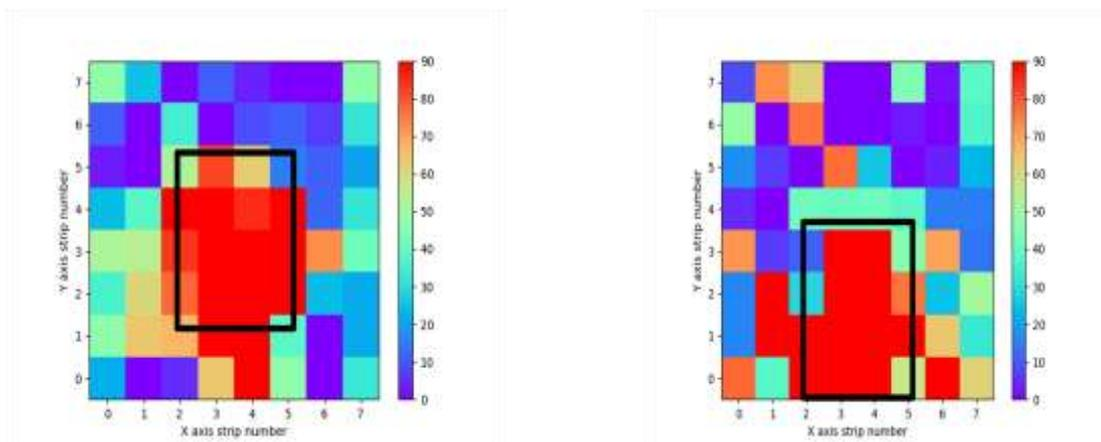
**Figure 8.** The images of the lead block as produced by the FPGA based DAQ
