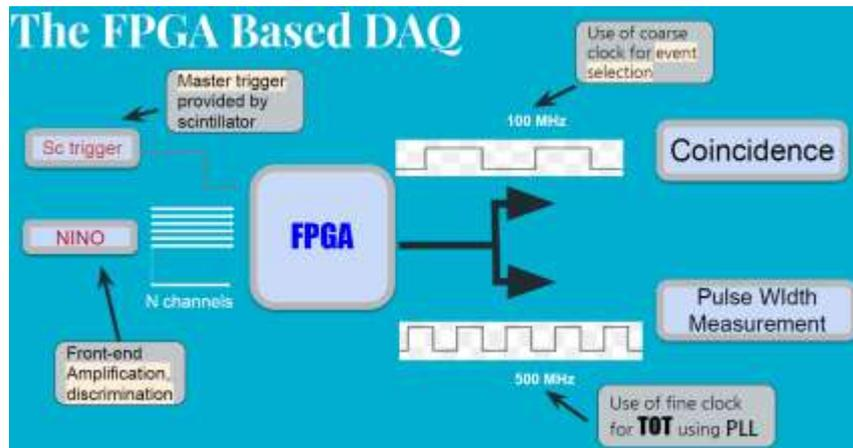
**Figure 6.** Schematic diagram of the FPGA based DAQ
