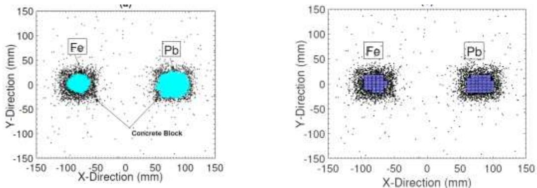
**Figure 4.** Images processed with DBSCAN (left) and PRM (right)
