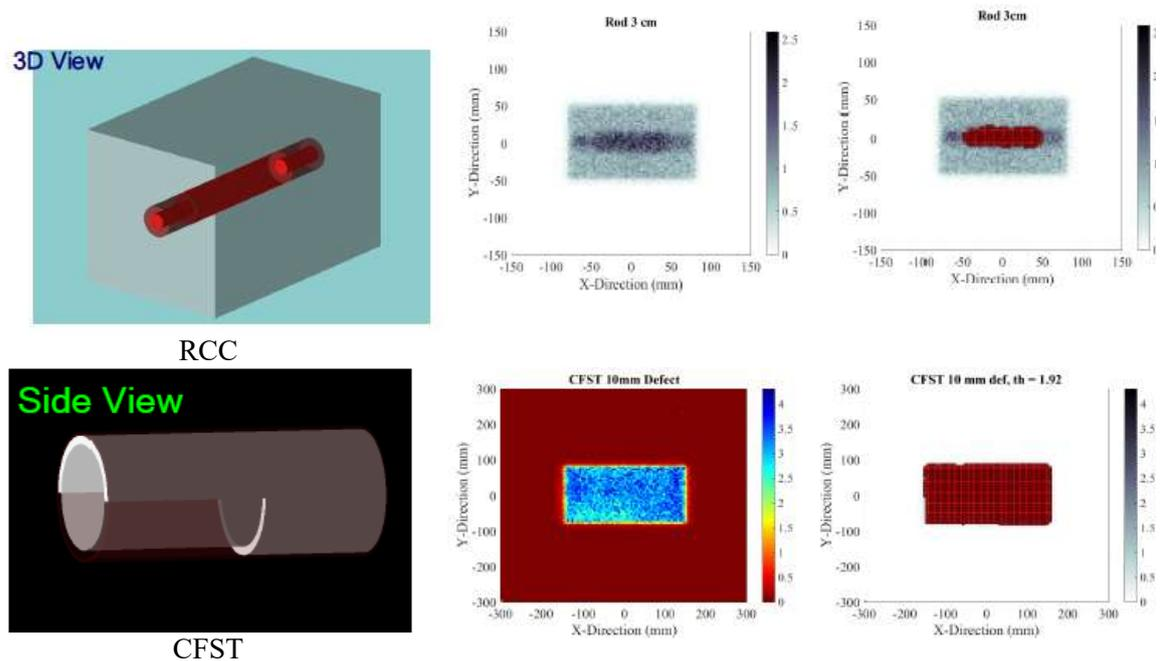
**Figure 5.** The two test models (left) of the civil structures, RCC and CFST along with their two dimensional projected images based on the scattering vertices (middle) and that after processing with the PRM (right)
