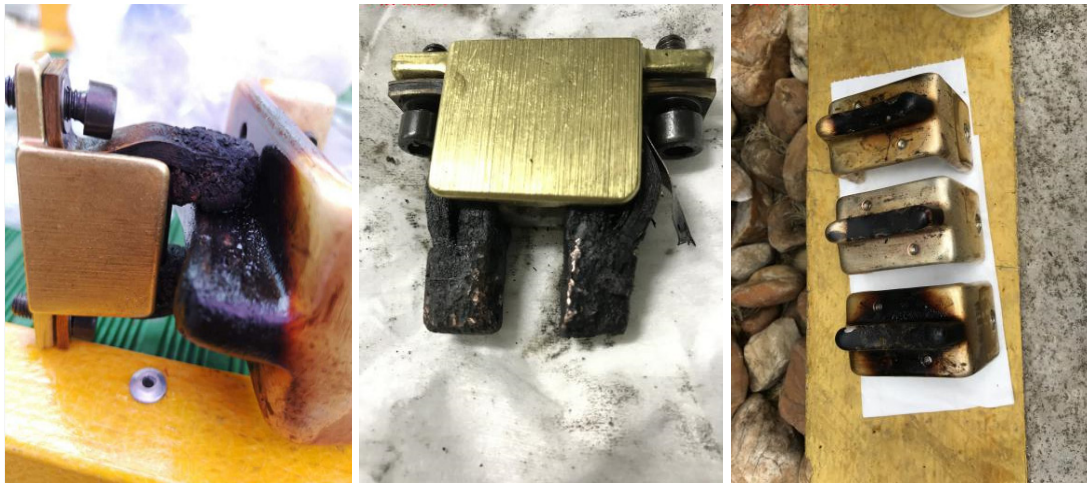
Figure 2 Main transformer A and B phase no-load tap changer dynamic and static contacts
