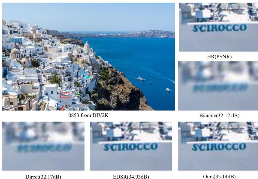
Figure 4 Comparison of PSNR of reconstructed images with different algorithms.
