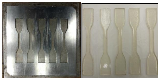
Figure 1. Dog-bone shaped mould according to ASTM D638
