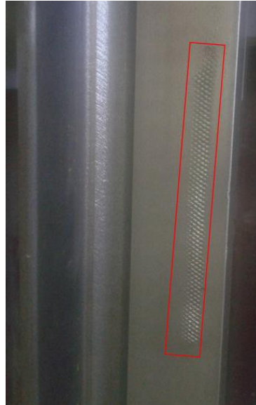
Figure 3. View with plastic damage on the guide rail working surface [8].
