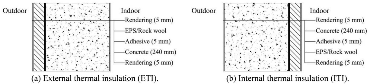
Figure 1. Thermal insulation configurations.
