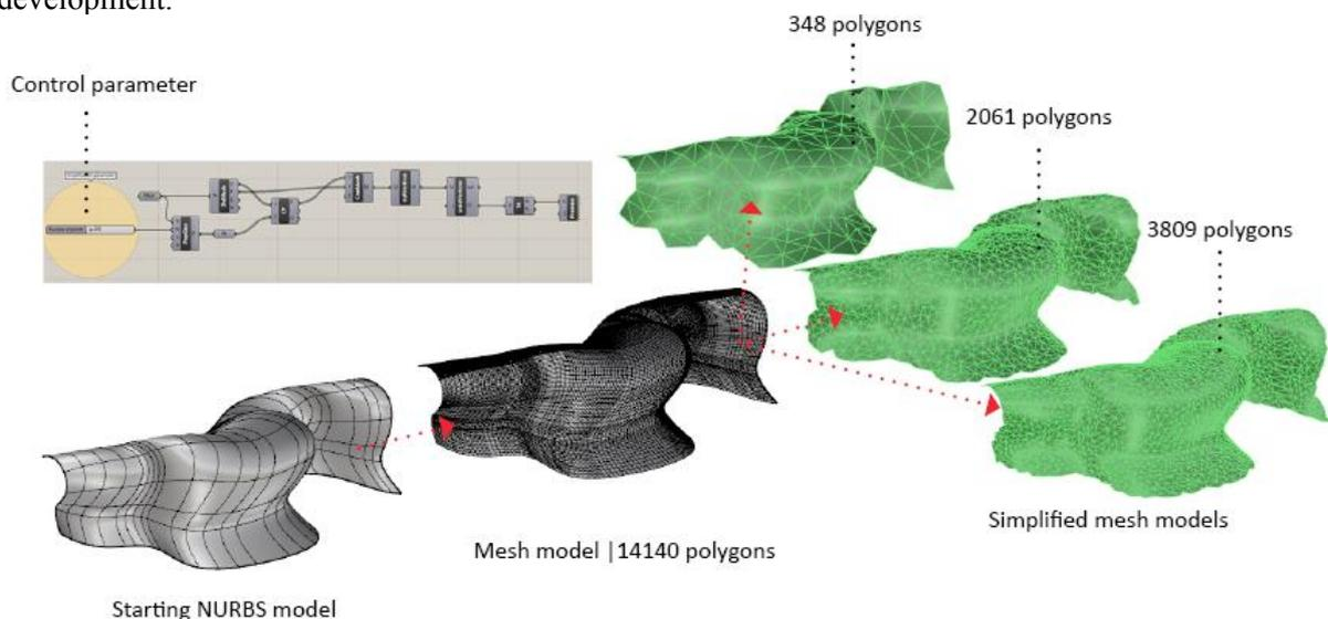
**Figure 2.** Schematic structure on a sample surface of the mesh simplification algorithm adopted.
