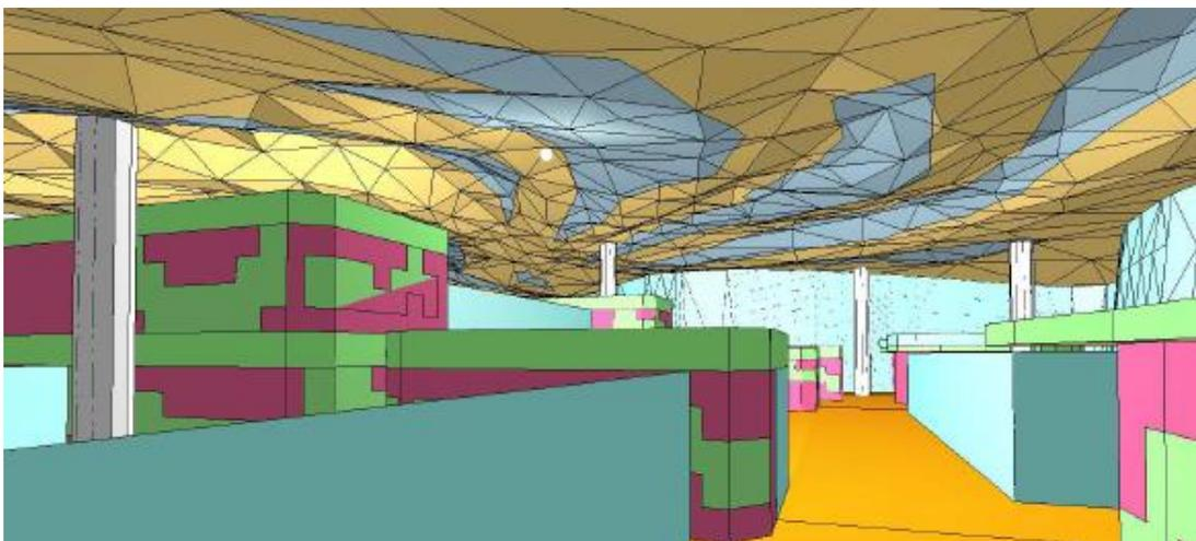
**Figure 5.** Internal view of the model in CATT-Acoustic with sound absorbing characteristics.
