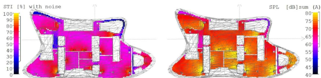
**Figure 7.** Maps of the STI (left) and Sound Pressure Level (right) in the final acoustic model.
