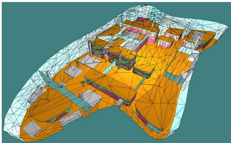
**Figure 1.** View of the model realized in CATT-Acoustic.
