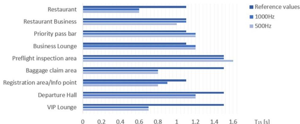
**Figure 6.** Reverberation time results for each terminal area.
