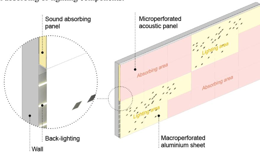
**Figure 4.** Sample box elevation and schematic view of acoustic and lighting surface interaction.
