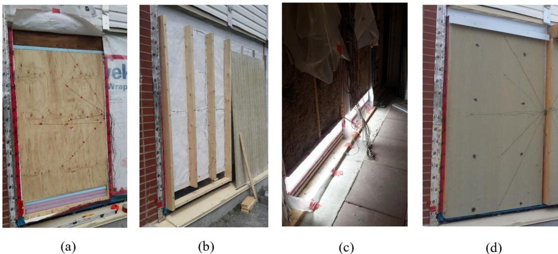
**Figure 3.** Experimental setup and sensor layout at different stages (a) thermistor installation on the sheathing layer (b) installation of weather barrier and strappings (c) wall opening viewed from the interior (d) thermistor installation on the cladding layer.
