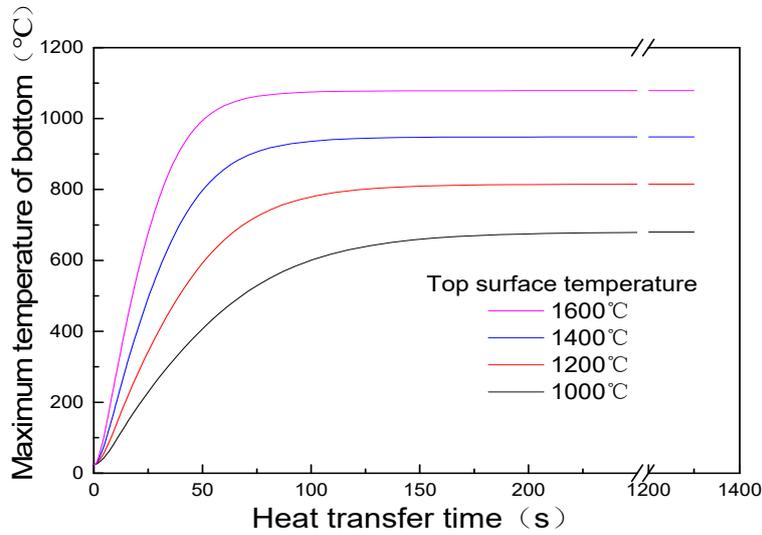
Fig.6 Curve of maximum temperature of bottom over time without heat insulation material
