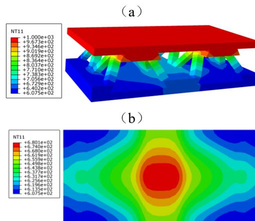
Fig.4 Temperature distribution without heat insulation material (a)overall structure (b)bottom
