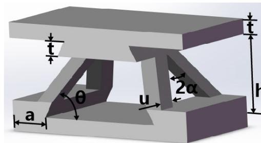
Fig.1 Unit cell of lattice structure
