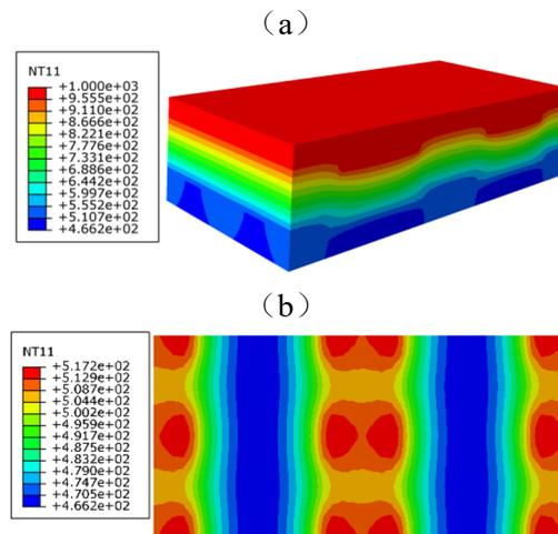
Fig.5 Temperature distribution with heat insulation material (a)overall structure (b)bottom
