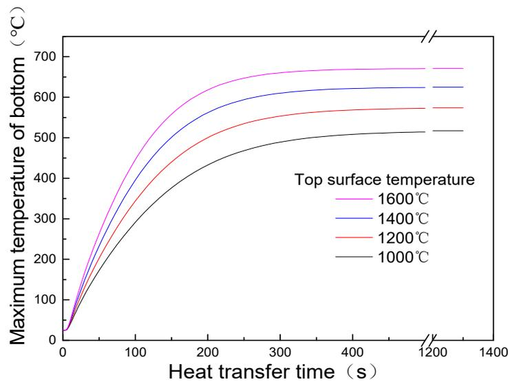
Fig.7 Curve of maximum temperature of bottom over time with heat insulation material
