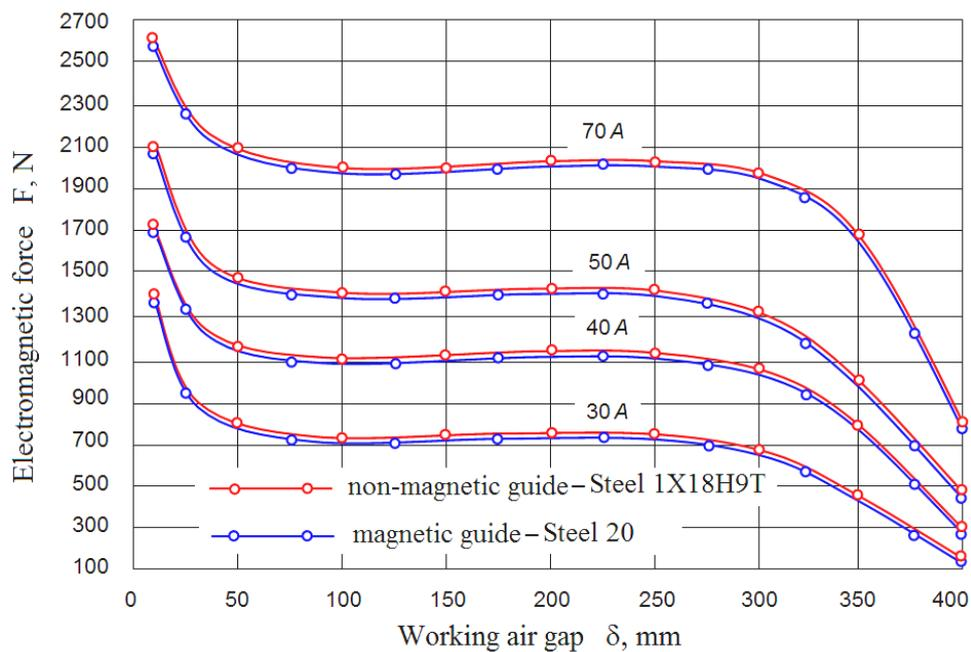
**Figure 5.** Static electromagnetic forces of the solenoid electromagnets with the shielding magnetic shell made of various materials
