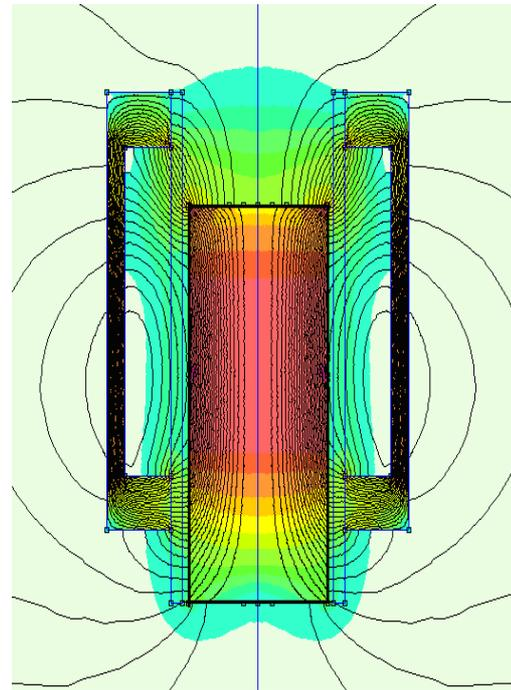
**Figure 4.** Magnetic flux lines in the solenoid with a shielding non-magnetic shell
