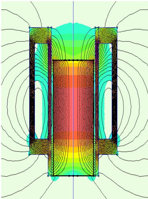
**Figure 3.** Magnetic flux lines in the solenoid with a shielding magnetic shell
