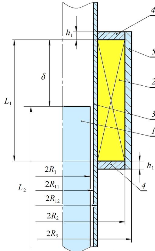
**Figure 2.** Design diagram of the solenoid electromagnet :
