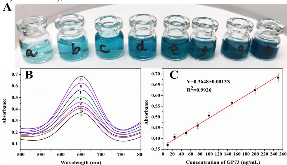
Figure 3. (A) Experimental phenomenon of different concentrations of GP73; (B) Absorbance curve of different concentrations of GP73; (C) Standard curve of GP73 at different concentrations
