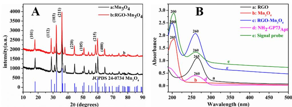
Fig.1 (A) XRD characterization of  $\text{Mn}_3\text{O}_4$  (curve a), RGO- $\text{Mn}_3\text{O}_4$  (curve b); (B) UV-vis characterization of RGO (curve a),  $\text{Mn}_3\text{O}_4$  (curve b), RGO-  $\text{Mn}_3\text{O}_4$  (curve c),  $\text{NH}_2\text{-GP73}$ (curve d), Signal probe (curve e)
