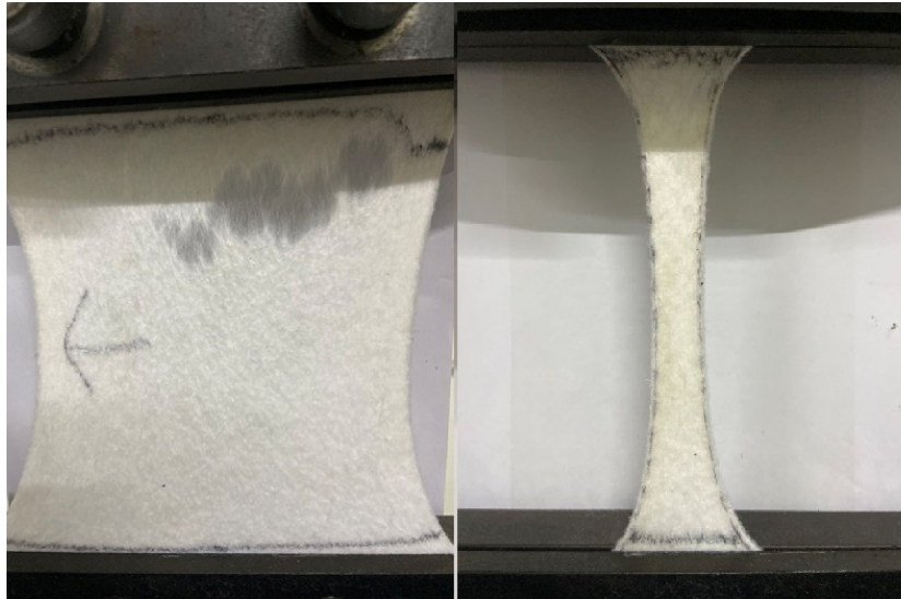
Figure 2 Comparison of test methods for tensile properties of Geotextiles
