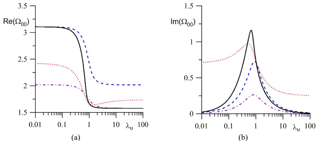
**Figure 2.** Frequency (a) and damping ratio (b) of volume natural oscillations vs wetting parameter  $\lambda_u$  for  $\Omega_{00}$  ( $R_0 = 5$ ,  $P_0 = 5$ ,  $b = 1$ ) (9).
