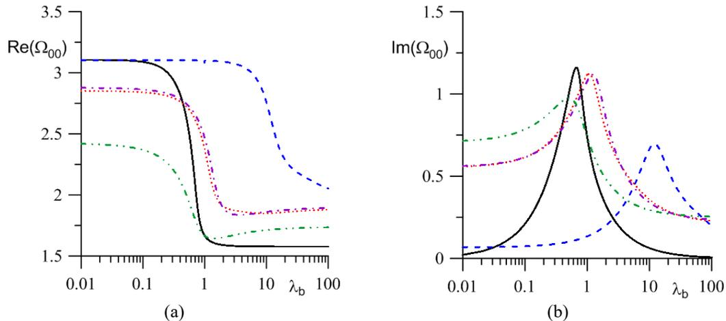
**Figure 3.** Frequency (a) and damping ratio (b) of volume natural oscillations vs wetting parameter  $\lambda_b$  for  $\Omega_{00}$  ( $R_0 = 5$ ,  $P_0 = 5$ ,  $b = 1$ ,  $\lambda_u = 1$ ).
