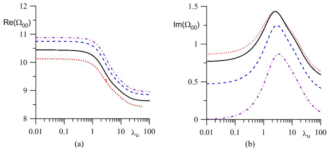
**Figure 5.** Frequency (a) and damping ratio (b) of volume natural oscillations vs wetting parameter  $\lambda_u$  for  $\Omega_{00}$  ( $R_0 = 5$ ,  $P_0 = 5$ ,  $b = 3$ ,  $k_\lambda = 1$ ).
