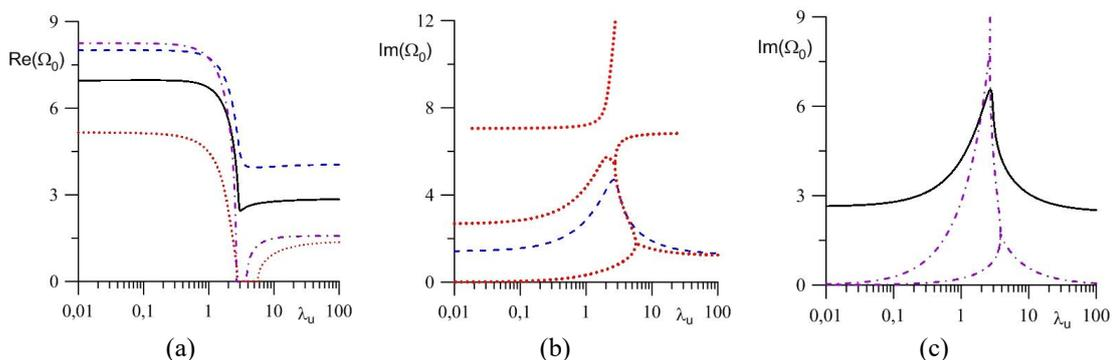
**Figure 4.** Frequency (a) and damping ratio (b, c) of volume natural oscillations vs wetting parameter  $\lambda_u$  for  $\Omega_{00}$  ( $R_0 = 5$ ,  $P_0 = 5$ ,  $b = 3$ ) (9).
