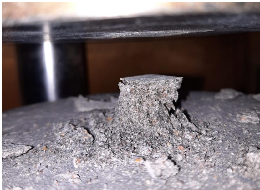
Figure 3. Fine-grained concrete after tests of the determination compressive strength.
