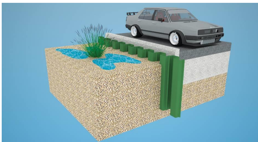
Figure 6. Vinyl sheet pile applied as Cut-off wall to protect construction of road
