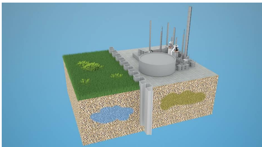
Figure 5. Cut-off walls in ecologically threatened areas
