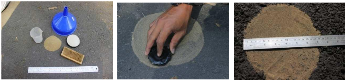
Figure 2. Sand Patch test for texture depth measurement
