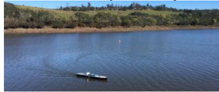
Figure 3. The turning circle test of 'Hoorn' in open water with diameter at 5.7*L .
