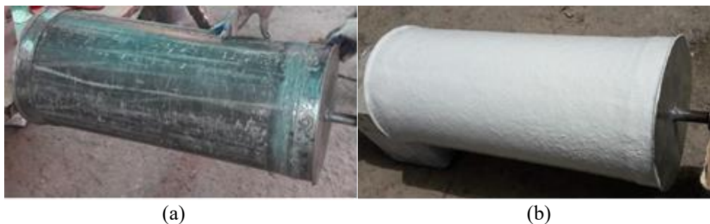
Figure 1. (a) Manufactured drum, (b) First coating layer with polyester resin on fiberglass and before polishing.
