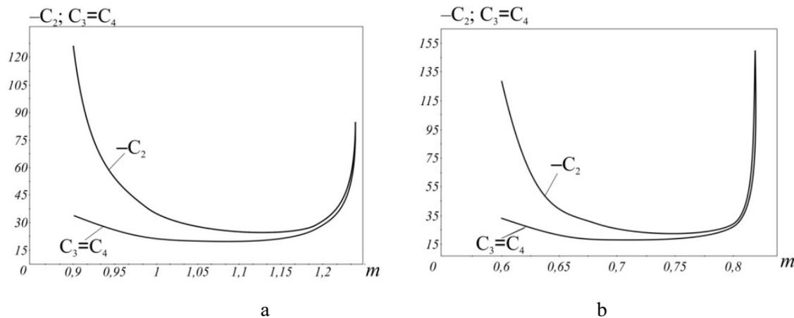
**Figure 2.** Graphs of coefficient functions  $C_1 - C_4$  with different  $m$  values and  $\frac{l_0}{l}$  for bending the workpiece by two equal forces: a -  $\frac{l_0}{l} = 0.15$ ; b -  $\frac{l_0}{l} = 0.20$
