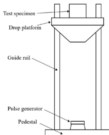
**Figure 1.** Model of the drop tower.
