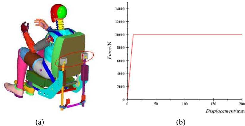
**Figure 3.** Simplified seat model and force-displacement curve of the energy absorbing element.
