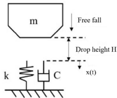
**Figure 6.** Schematic diagram of the drop tower.
