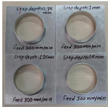
**Figure 6** Hole flanges formed using SPIF to study effect of step depth
