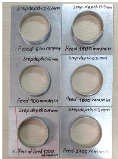
**Figure 3** Hole flanges formed using SPIF to study effect of feed
