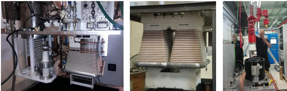
**Figure 4.** RF generator during assembly.
