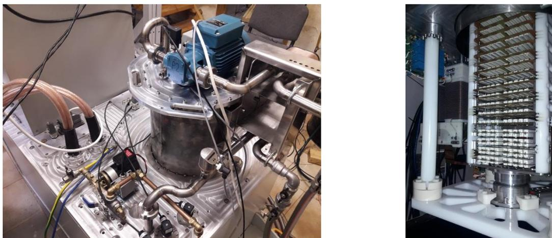
**Figure 5.** The dual equivalent resistive load: top part of the load over the tank cover – on the left, bottom part of the load under the tank cover – on the right.
