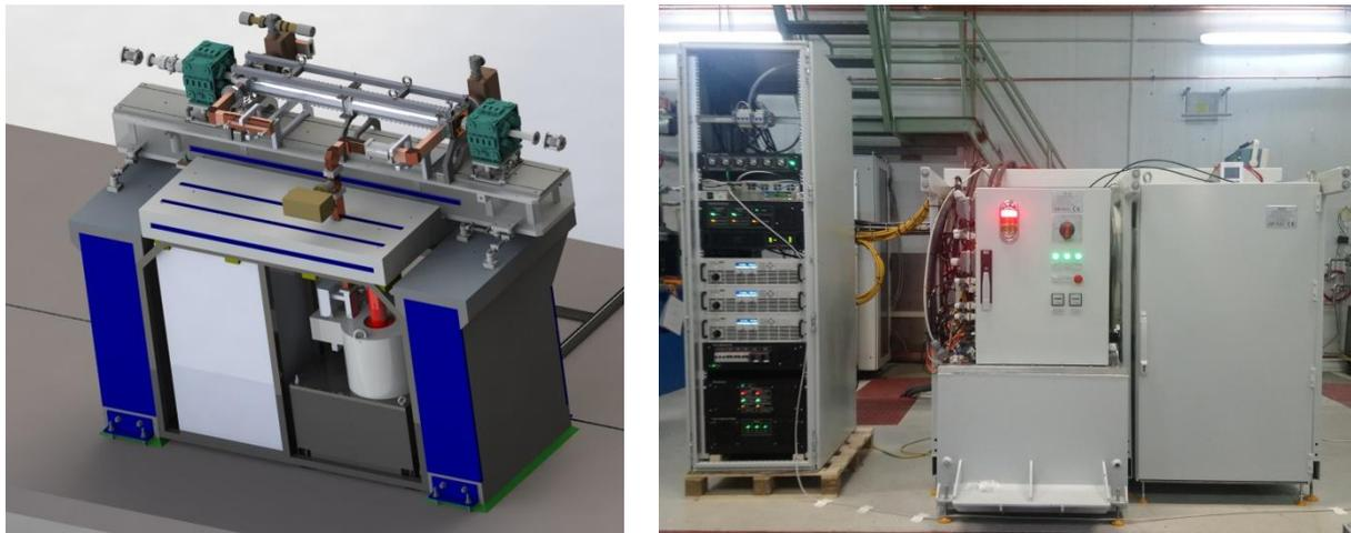
**Figure 1.** 3D design of the transverse deflecting system TDS BC1 (left) and the system at the DESY test stand (right).
