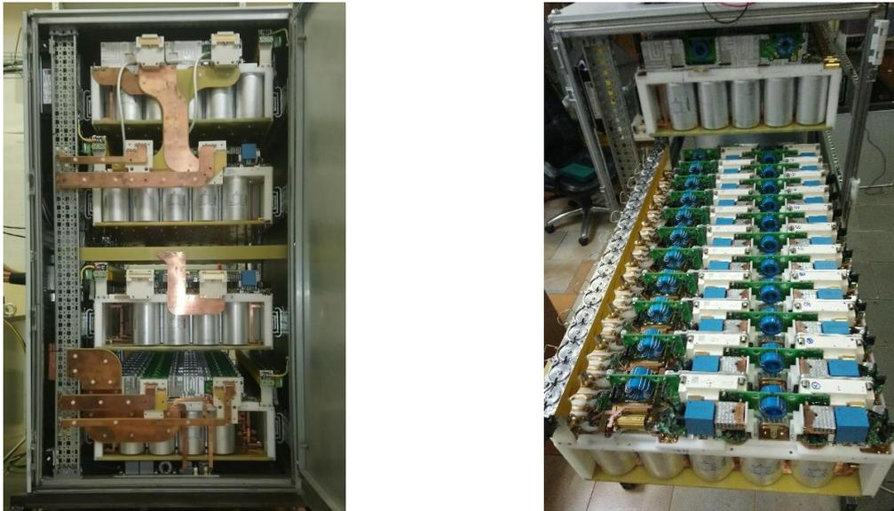
**Figure 3.** Modulator (left) and 11 kV module (right).
