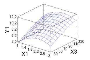
**Figure 4**. The response surface of the output parameter sulfur content wt.%  $Y_1$  from variable factors - the ratio SAA: U  $X_1$  and the duration of the process  $X_3$  with the ratio SC: St 1:4.
