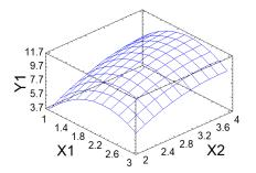
**Figure 2.** The response surface of the output parameter sulfur content wt.% Y1 from variable factors - the ratio of SAA:U  $X_1$ , the ratio of St:SC  $X_2$ , with a duration of 120 minutes.
