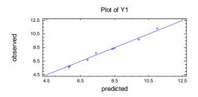
Figure 3. Comparison of experimental and calculated values of sulfur content in sulfated starch during sulfation with varying SAA: U ratio and process duration.
