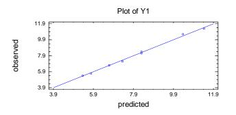
**Figure 5.** Comparison of experimental and calculated values of sulfur wt% in a sulfated starch sample during sulfation with varying SC: St ratio and process duration.
